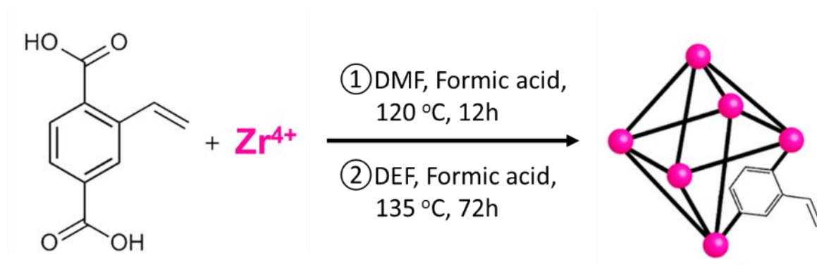
Figure 3.2. Schematic synthesis of olefin substituted Zr-MOF in bulk crystalline powders by route ① and single crystals suitable for SCXRD by route ②.
