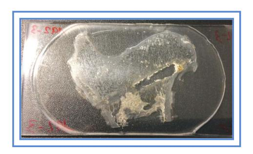
Figure 32: Final aspect of the sheet once polished up to 50-100 micrometers of diameter.
