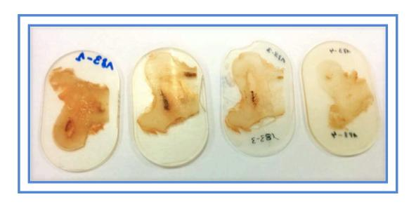
Figure 31: Images of the solid blocks of PMMA resin with the bone samples inside.
