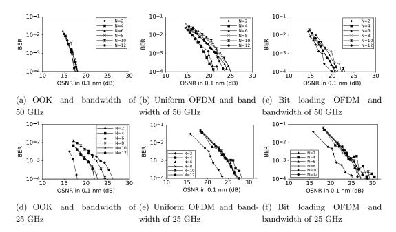
Figure 4.7: BER vs OSNR for the OOK approach (a and d), DD-OFDM approach using uniform loading (b and e) and bit loading (c and f) after cascade filters with bandwidths of 50 GHz (a, b, c) and 25 GHz (d, e, f).
