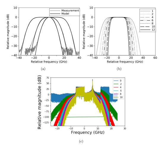
Figure 4.3: (a) Model fitting of the filter for bandwidths of 12.5 GHz, 25 GHz and 50 GHz. (b) Transfer function when concatenating up to 12 times the transfer function of a 50 GHz filter. (c) Optical spectrum of the OFDM signal after being affected by several filter stages.
