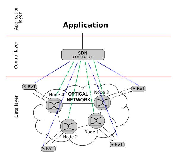
Figure 2.2: Generic Software Defined Network (SDN) architecture. S-BVT: Sliceable-Bandwidth Variable Transceiver.
