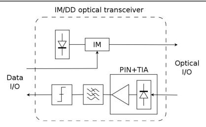
Figure 4.1: IM/DD OOK transceiver scheme. I/O: Input/Output, IM/DD: Intensity Modulation/Direct Detection.
