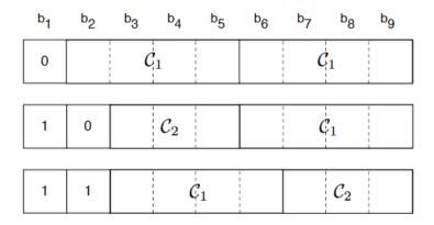
Figure 6.1: Bit-to-symbol mapping for 6PQPSK.  $C_1$  corresponds to the DPQPSK constellation format and  $C_2$  corresponds to PSQPSK format.
