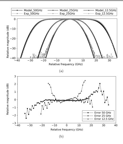
Figure 4.6: (a) Model fitting of the experimental filter characterization for bandwidths of 12.5 GHz, 25 GHz and 50 GHz. (b) Relative error between the model and the experimental filter characterization for bandwidths of 12.5 GHz, 25 GHz and 50 GHz.
