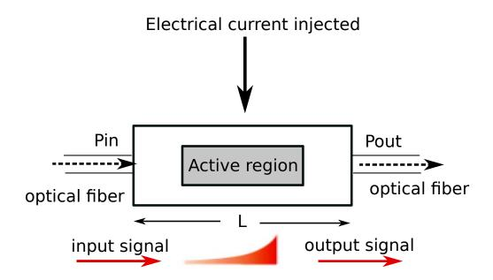
Figure 5.2: Semicondutor Optical Amplifier (SOA) structure. Pin: input power, Pout: output power, L: length.
