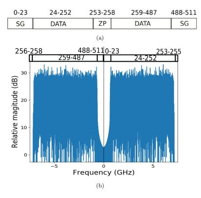
Figure 6.5: a) Frame structure for 512 subcarriers and b) its corresponding mapping in frequency domain. ZP: Zero padding, SG: Spectral Gap.
