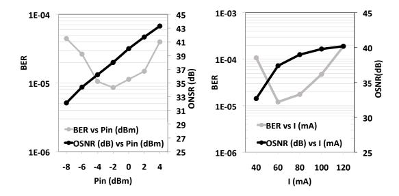
Figure 5.6: SOA characterization. (a) BER versus  $P_{in}$  (input power) and OSNR versus  $P_{in}$  for a fixed bias current of 65 mA. (b) BER versus I (SOA bias current) and OSNR versus I for a fixed  $P_{in}$  of -2 dBm.
