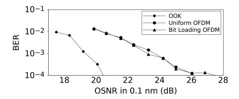
Figure 4.8: BER vs OSNR for the OOK approach, the DD-OFDM SSB approach using uniform loading and bit loading after 2 filters with bandwidths of 12.5 GHz.
