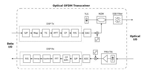
Figure 4.2: Optical OFDM transceiver scheme. TLS: Tunable Lightwave Source; MZM: Mach-Zehnder Modulator; S/P: Serial to Parallel, TS: Training Symbol insertion, CP: Cyclic Prefix, P/S: Parallel to Serial.
