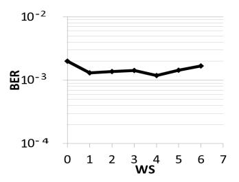
Figure 5.7: BER versus WS for 75 km of fiber and OSNR of 36 dB without considering SOAs placed inline. WS: Window Size.
