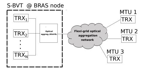
Figure 3.3: Generic architecture for BRAS-MTU connectivity. MTU: MultiTenant Unit, BRAS: Broadband Remote Access Server. S-BVT: Sliceable-Bandwidth Variable Transceiver, TRX- Transceiver.
