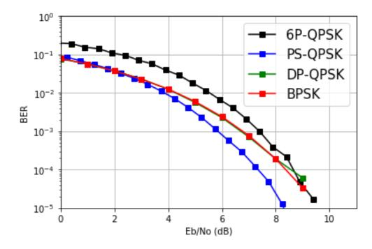
Figure 6.2: BER performance versus  $E_b/N_0$  for DPQPSK, PSQPSK, 6PQPSK and BPSK constellation formats.
