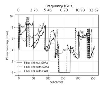
Figure 5.10: Power loading assignment considering MA at 28 Gb/s over two SSMF spans of 25 km, with and without SOAs and for SOAs-based OAD, at 34 dB of OSNR.
