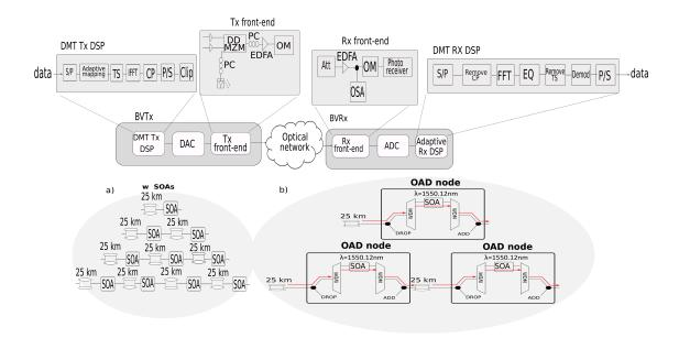
Figure 5.4: S-BVT architecture and experimental set-up. OM: optical power monitoring, Att: Attenuator, OSA: Optical Spectrum Analyzer, EQ: Equalizer. The different analyzed scenarios for the optical metro network are indicated: a) with SOAs and 25km SSMF spools, and b) with OAD nodes based on SOAs.
