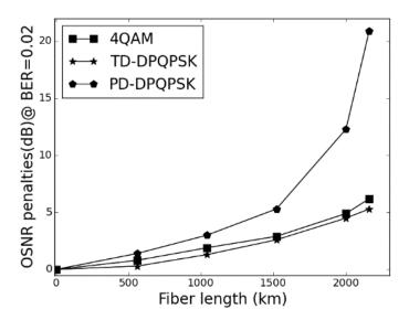
Figure 6.8: OSNR penalties at a target BER for different fiber lengths considering the transmission schemes of 4QAM, TD-DPQPSK and PD-DPQPSK.
