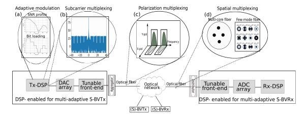
Figure 2.7: Multi-adaptive optical transceivers based on a) adaptive modulation, b) subcarrier multiplexing, c) polarization multiplexing and d) space division multiplexing (multi-core and few-mode fibers).
