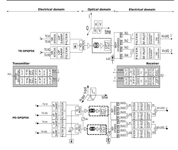
Figure 6.3: Block diagram for the TD-DPQPSK and PD-DPQPSK transmission schemes. MOD: Modulator, S/P: Serial to parallel, TS: Training Symbols, ZP: Zero Padding, SG: Spectral Gap, IQ: Inphase Quadrature, OPT FILT: Optical Filter, RF: Radio Frequency, FFT2D: Fast Fourier Transform 2 Dimensions, IFFT2D: Inverse Fast Fourier Transform 2 Dimensions.
