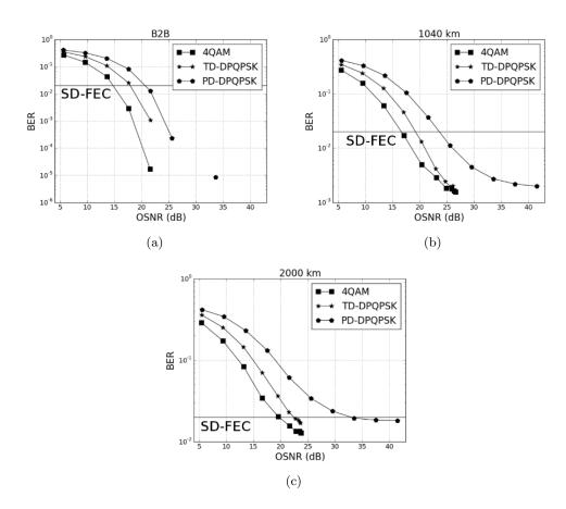
Figure 6.7: BER vs OSNR for 4QAM, TD-DPQPSK and PD-DPQPSK for a) B2B, and after b)1040 km and c)2000 km of fiber.
