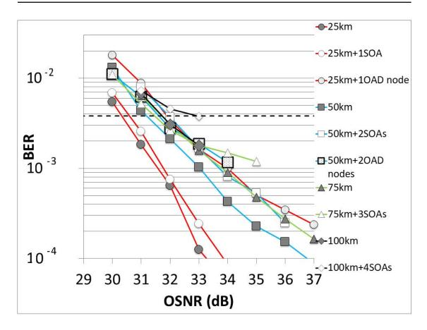
Figure 5.13: BER versus OSNR (with and without SOAs and including SOA-based OAD nodes) using bit and power loading algorithms under the MA criteria for a fixed gross bit rate of 28 Gb/s.
