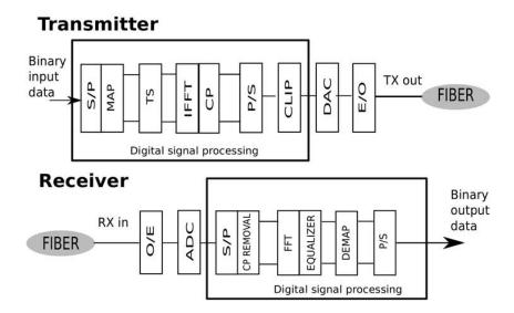
Figure 2.4: Conceptual diagram of a generic OFDM system. S/P:Serial to Parallel, MAP: MAPping, TS: Training Symibols, IFFT: Inverse Fast Fourier Transform, CP: Cyclic Prefix, P/S: Parallel to Serial, CLIP: CLIPing, DAC: Digital to Analog Converter, E/O: Electrical to Optical, O/E: Optical to Electrical, ADC: Analog to Digital Converter, S/P: Serial to Parallel, FFT: Fast Fourier Transform, DEMAP: DEMAPping, P/S: Parallel to Serial.
