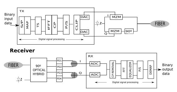
Figure 2.6: CO-OFDM transmitter and receiver.
