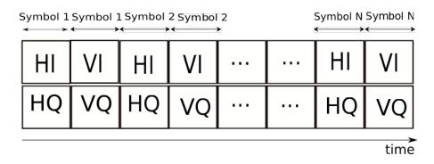
Figure 6.4: Interleaving of the polarization signals in time dimension. HI: Horizontal Inphase, HQ: Horizontal quadrature, VI: Vertical Inphase, VQ: Vertical Quadrature.
