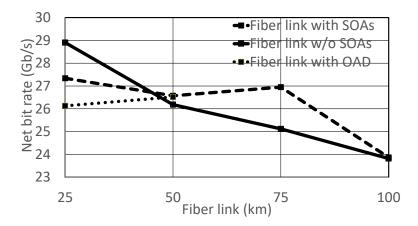
Figure 5.14: Net bit rate versus fiber link (with and without SOAs and including SOA-based OAD nodes), using RA bit and power loading algorithms, for an OSNR of 33 dB at target BER of  $3.8 \cdot 10^{-3}$ .
