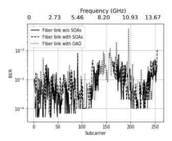
Figure 5.11: BER per DMT subcarrier considering MA at 28 Gb/s over two SSMF spans of 25 km, with and without SOAs and for SOAs-based OAD, at 34 dB of OSNR.
