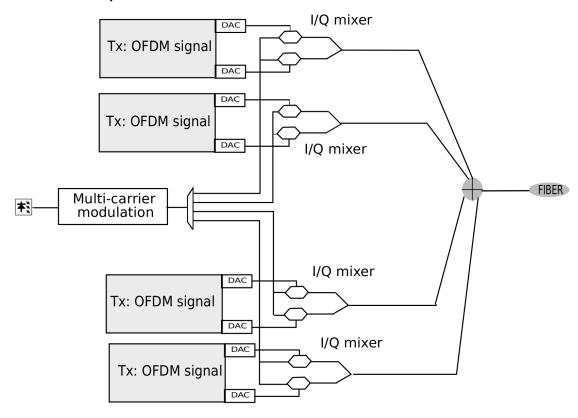
Figure 2.8: Multi-band OFDM transmitter based on (a) electrical I/Q Mixers and in (b) optical I/Q mixers.
