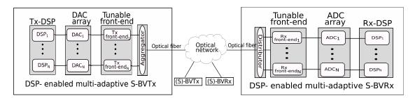
Figure 2.3: Generic S-BVT architecture. DSP: Digital Signal Processing, DAC: Digital to Analog Converter, ADC: Analog to Digital Converter, SNR: Signal to Noise Rate, Tx: Transmitter, Rx: Receiver.
