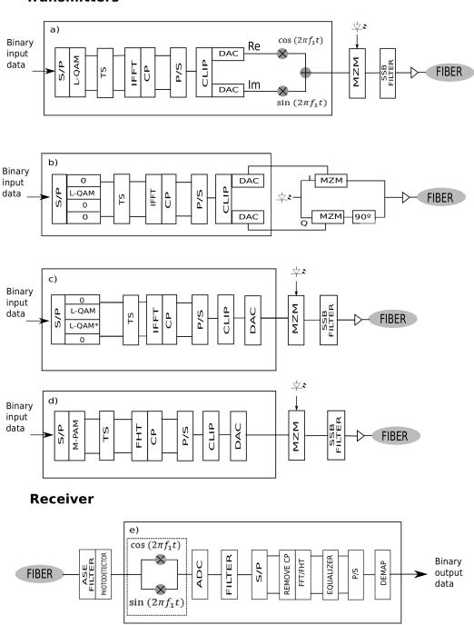
Figure 2.5: DD-OFDM transmitters using a) RF upconverter and optical SSB filter, b) frequency domain Hilbert transform, c) Hermitian symmetry and an optical SSB filter, d) real transform (DHT) and an optical SSB filter and e) DD-OFDM receiver. SSB:Single Side Band, MZM: Mach-Zhender Modulator, ASE: Amplified Spontaneous Emission.
