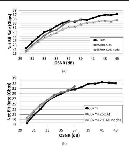
Figure 5.15: Net bit rate versus OSNR for (a) 25 km and (b) 50 km for the different scenarios at the target BER.
