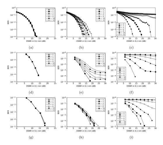
Figure 4.4: Simulation results for a standard IM/DD system (a, b, c), the OFDM SSB transceiver (d, e, f), the OFDM SSB transceiver using bit loading (g, h, i) after concatenation of different filters featuring bandwidths of 50 GHz (a, d, g), 25 GHz (b, e, h) and 12.5 GHz (c, f, i).
