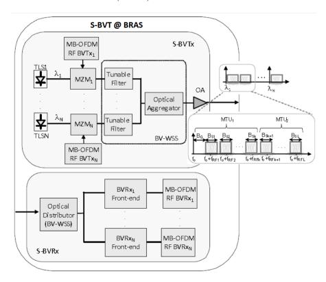
Figure 3.4: S-BVT sited at the BRAS. WSS: wavelength selective switch, MB: Multi-Band, S-BVTx: Sliceable-Bandwidth Transceiver at the transmitter. S-BVRx: Sliceable-bandwidth Transceiver at the Receiver. MTU: MultiTenant Unit.
