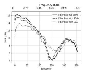
Figure 5.8: SNR profile considering MA at 28 Gb/s over two SSMF spans of 25 km, with and without SOAs and for SOAs-based OAD, at 34 dB of OSNR.
