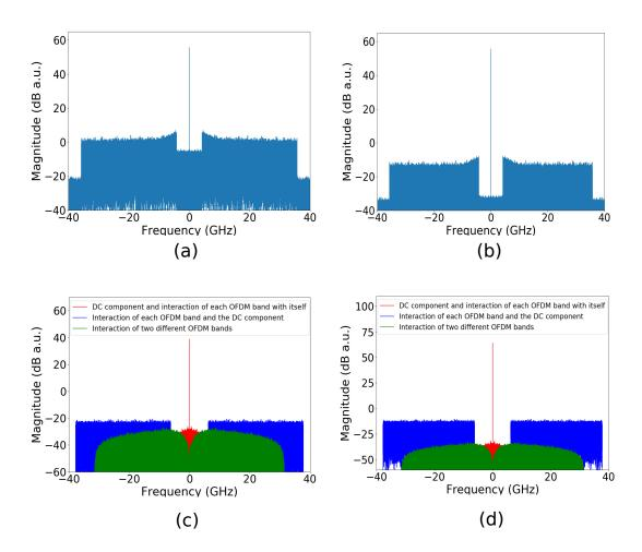
Figure 3.2: Signal spectrum after the photodetector with a MZM biased (a) near the null point  $(V_{bias}/V_{\pi}=0.9)$  and (b) near the quadrature point  $(V_{bias}/V_{\pi}=0.6)$  for a B2B system. Frequency distribution of the different contributions in (3.16) with the MZM biased (c) near the null point  $(V_{bias}/V_{\pi}=0.9)$  and (d) near the quadrature point  $(V_{bias}/V_{\pi}=0.6)$
