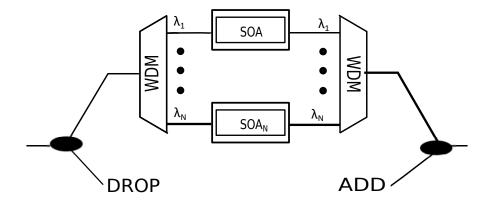
Figure 5.3: Estructure of an OAD node.SOA: Semiconductor Optical Amplifier, WDM: Wavelength Division Multiplexing.
