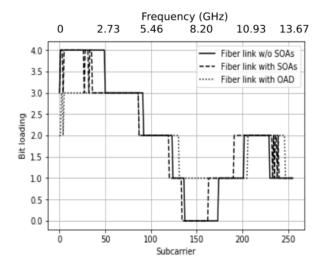
Figure 5.9: Bit loading assignment considering MA at 28 Gb/s over two SSMF spans of 25 km, with and without SOAs and for SOAs-based OAD, at 34 dB of OSNR.
