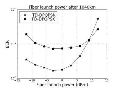
Figure 6.6: BER versus fiber launch power after 1040km of fiber for TD-DPQPSK and PD-DPQPSK transmission schemes.
