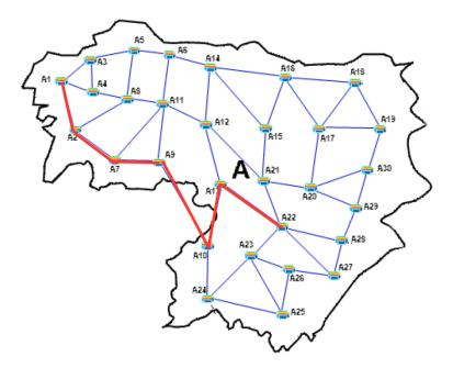
Figure 3.5: Region-A of the Telefonica Spanish network. The considered path traverses the nodes 1, 2, 7, 9, 10, 13 and 22 for a maximum length of 545km.
