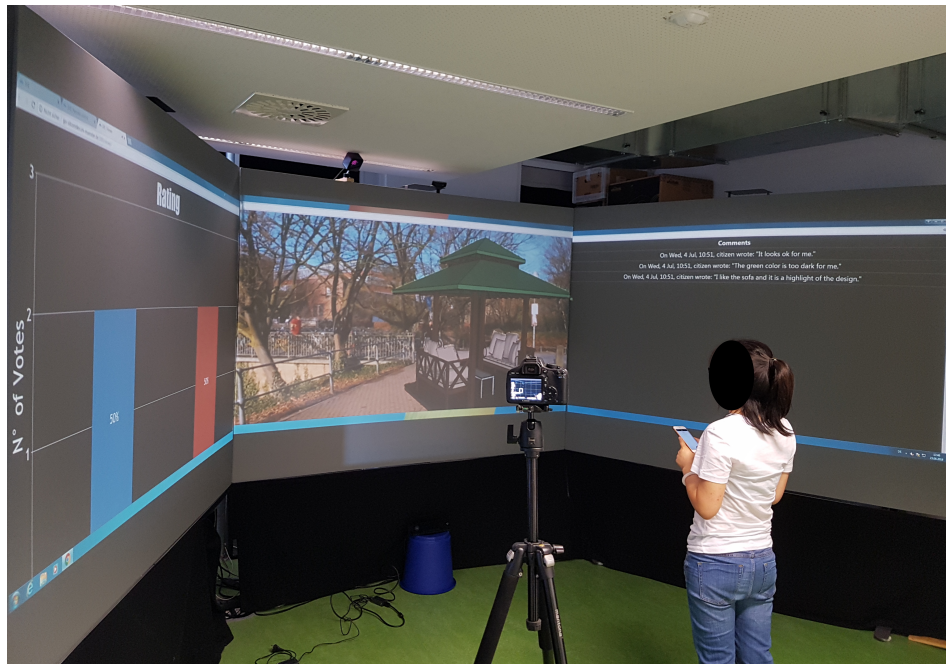
Fig. 5.1: Prototypical implementation of the proposed approach: immersive video environment consisting of three large screens; central screen shows panoramic video and planned building; side screens show voting results and comments; user votes/comments using simple web app on mobile phone.
