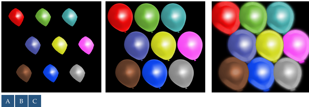
FIGURE 6.1: Soft color erosion (A), the L^*a^*b^* -encoded Balloons image (B) and soft color dilation (C), with the minimum t-norm, its residual implication (the Gödel implication) and a 31 \times 31 -pixel Gaussian-shaped structuring element, with \sigma = 8 pixels and a maximum value of 1. We remark that the irregular shapes of the eroded balloons reflect their irregular illumination.
