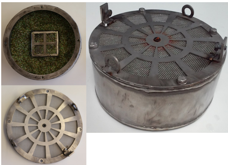
Fig. 2. New underdrain built and filled with 0.85–1.50 mm crushed recycled glass.
