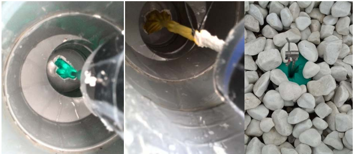
Figure 2.23- Fastening system and isolation of the ADV with a balloon.
