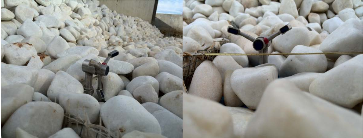
Figure 2.8- ADV placement on the bed surface.
