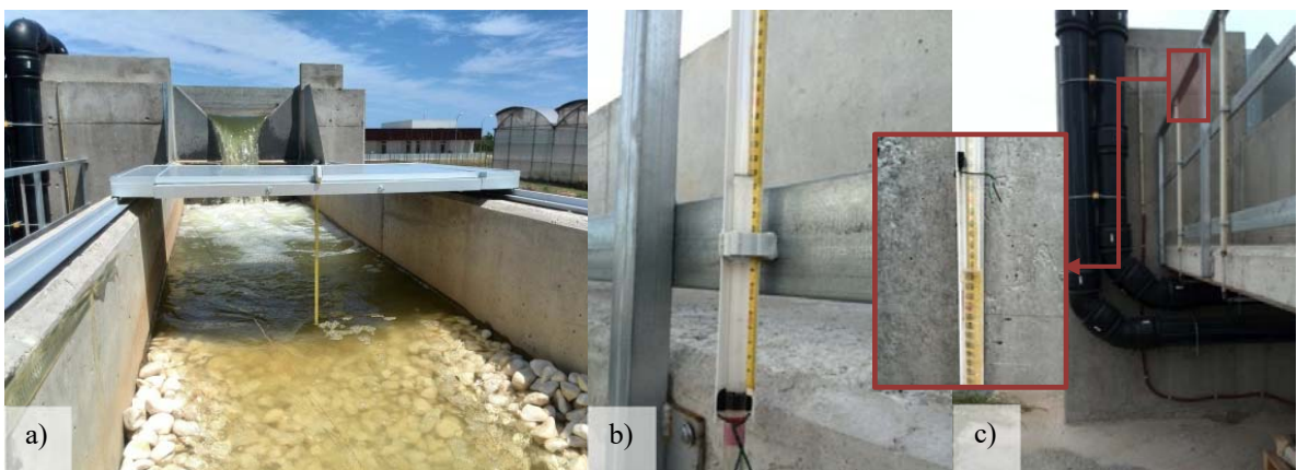
Figure 2.5- Water depth measurements (a) water level gauge, (b) channel piezometer and (c) spillway tank piezometer.
