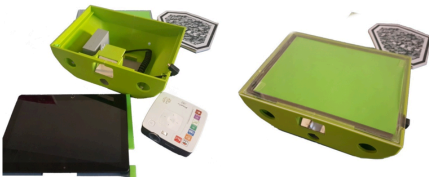
Figure 35. Functional WaS prototype based on a marker-recognition system
