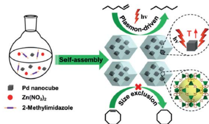
Figure 2.1. Synthesis scheme of the Pd nanocubes@ZIF-8 and the plasmon-driven photothermal effect used in hydrogenation reactions. 56
