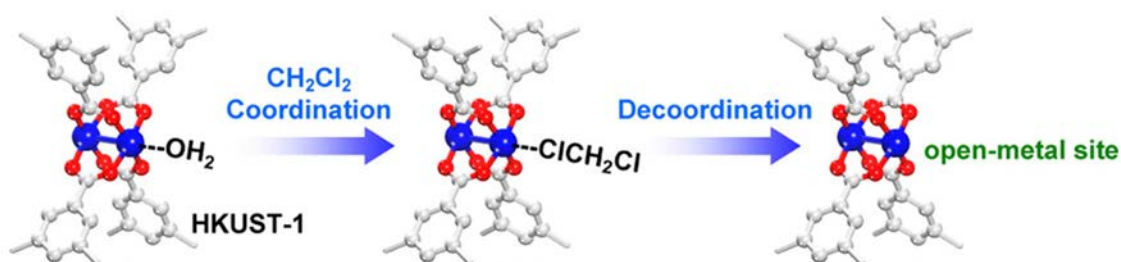
Figure 3.1. Schematic representation of the solvent exchange procedure in HKUST-1. 71
