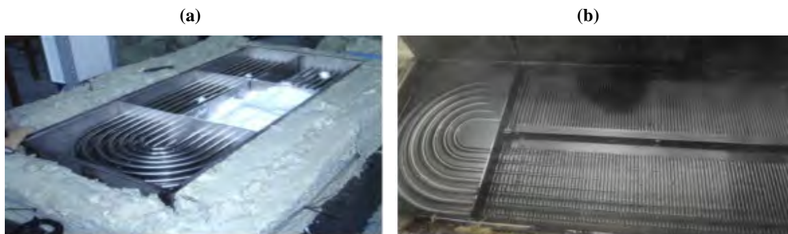
Fig. 5. (a) Storage TES system without fins. (b) Storage TES system with fins used in the experimentation [13].
