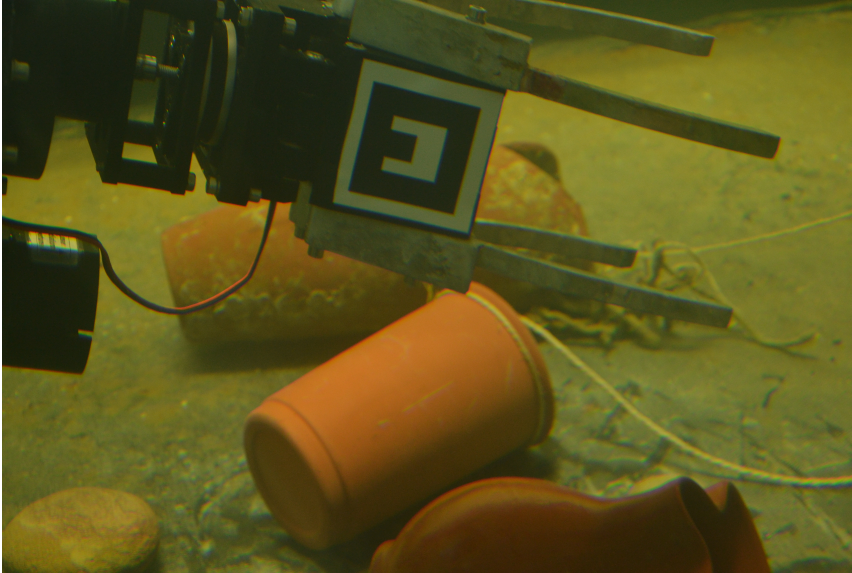
Figure 6.2: AR marker attached at the gripper of the ARM5E manipulator.
