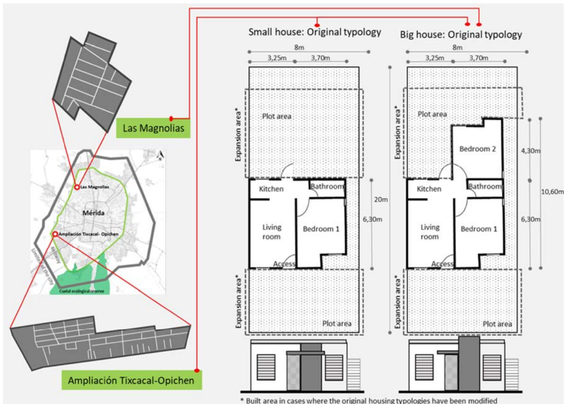
Figure 11.3 Urban plan of the two sample neighborhoods and dimensions and distribution of the two original typologies of social housing.
