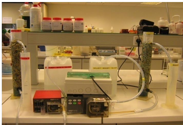
Figure 5.3. Two similar column set-ups for zeolite tests with larger particle grain size.
