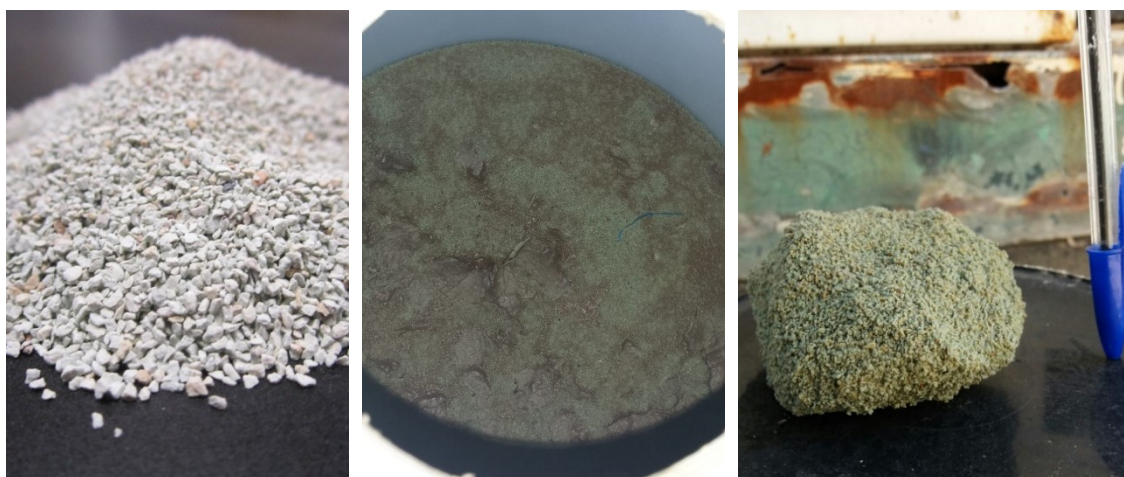
Figure 6.9. Sample of new zeolitic material used in this study (left), top view of the zeolite column after fourteen cycles (middle) and sample of a portion of the compacted column bed material after fourteen cycles of operation (right).
