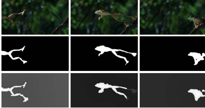
Figure 1.5 – Example of video saliency results. (top) input frames, (middle) ground truth and (bottom) video saliency results.
