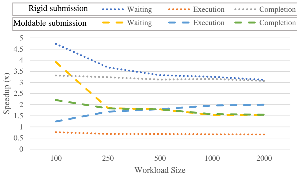
Figure 7.2: Comparison of the 4 types of workloads. The lines show the speedup of malleability for the average job waiting, execution, and completion time, grouped by submission mode.
