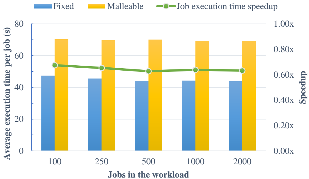
Figure 6.25: Average job execution time on different fixed and malleable workloads with an increasing number of jobs.
