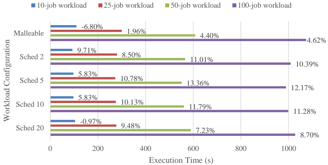
Figure 6.11: Execution time for the different inhibition periods (bars) and the gain respect the rigid workload (percentage on the right side of the bars) with synchronous scheduling.
