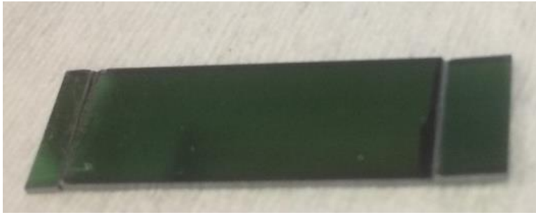
Figure 3.14 Sensor chip diced with a 2 mm single mode section followed by a 15 mm sensing area and 5 mm bimodal section. The chip was later polished and the microfluidic system was attached to repeat the calibration of the shorter biosensor.
