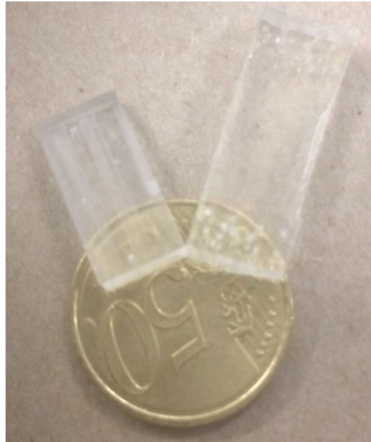
Figure 3.27 PDMS cells obtained after mould casting of the previous SU-8 chips.
