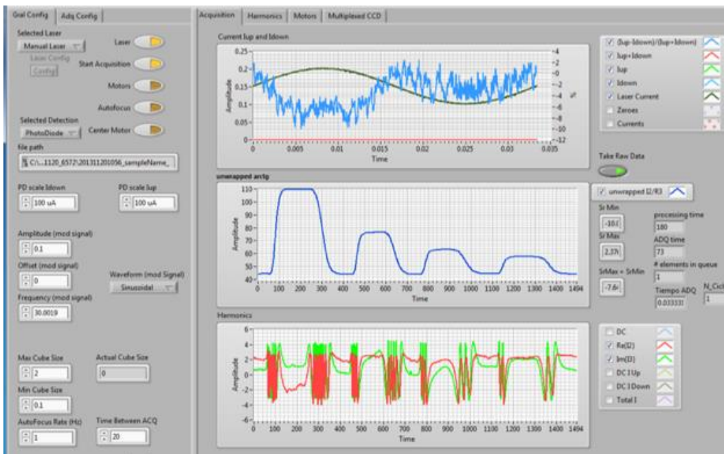
Figure 3.15 Bulk calibration of the short chip (total length of 22 mm). Injections of 0.5, 0.25, 0.15 and 0.10 M of HCl were successive performed.
