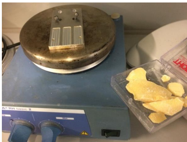
Figure 2.11 Chip holders and wax for polishing. They were heated in a plate at 90°C, then cooled down for polishing and re-heated for the chip removal.
