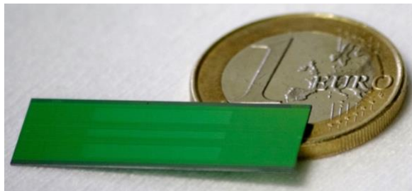
Figure 2.9 Photograph of a BiMW sensor chip after cleaning. Each chip includes three groups of 8, 4 and 8 BiMWs and has a total dimension of 3 x 1 cm.
