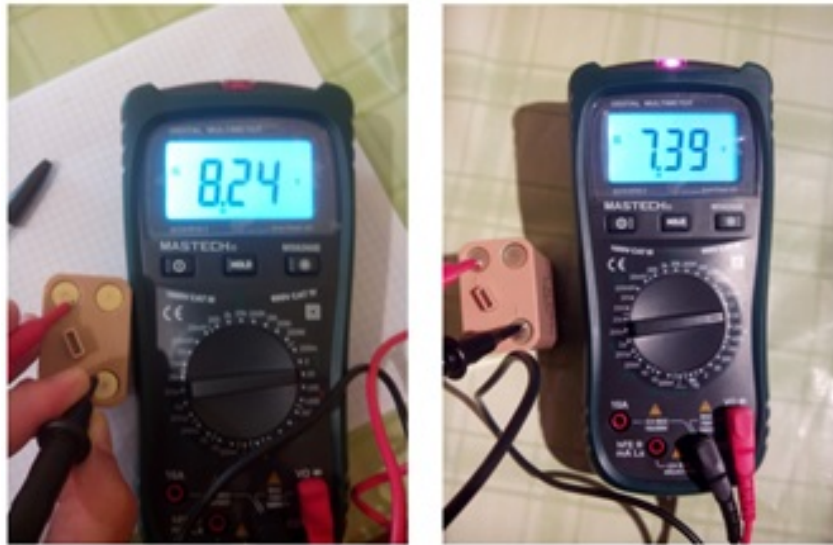
FIGURE 3.10: (Left) The battery works perfectly. (Right) Once Pleo has no power to make it run, its battery have exactly 7.39 V.
