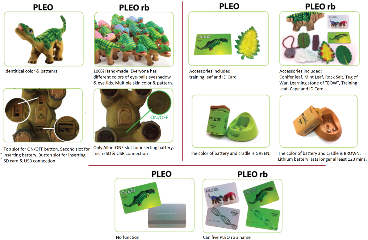
FIGURE 3.5: Main differences between Pleo and Pleo rb.
