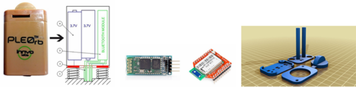
FIGURE 3.8: (Left) Layout of the proposed assembly; (Middle) Modules JY-MCU and RN-41; (Right) 3D print model.
