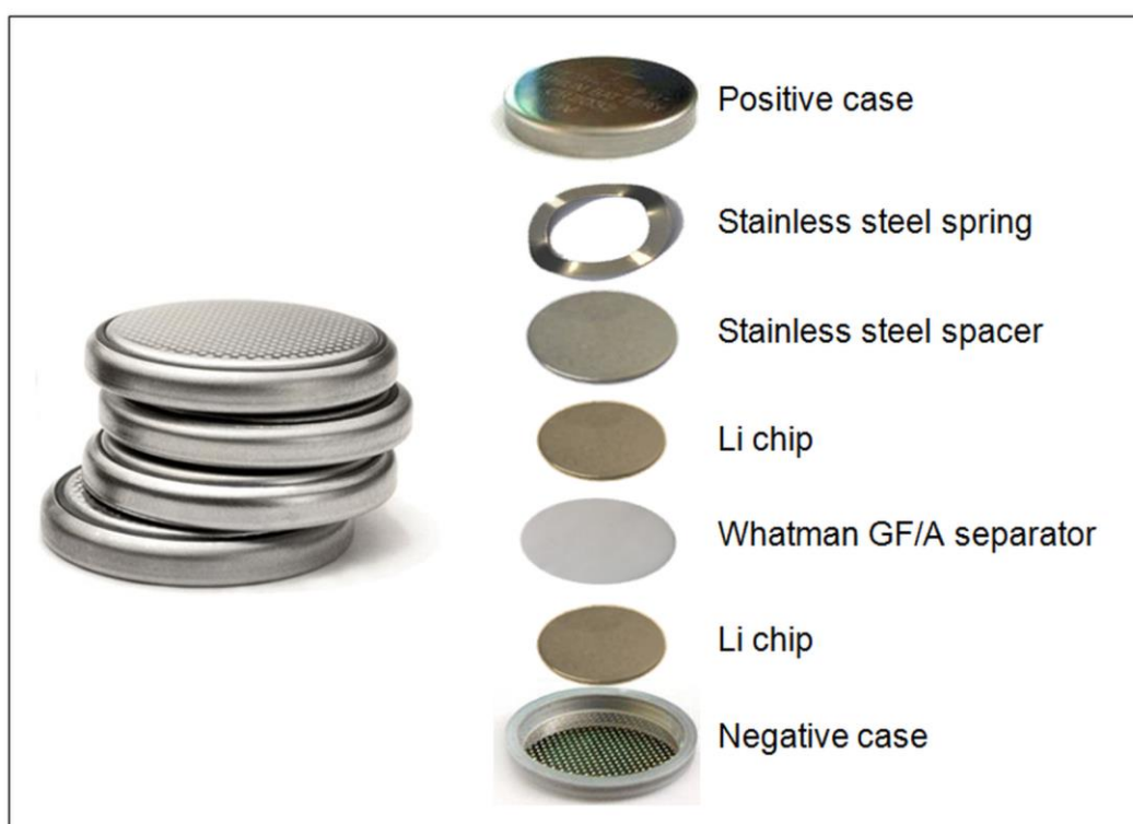
Figure 28: Photo of a CR2032 coin cell and its components for the Li stripping/plating test.
