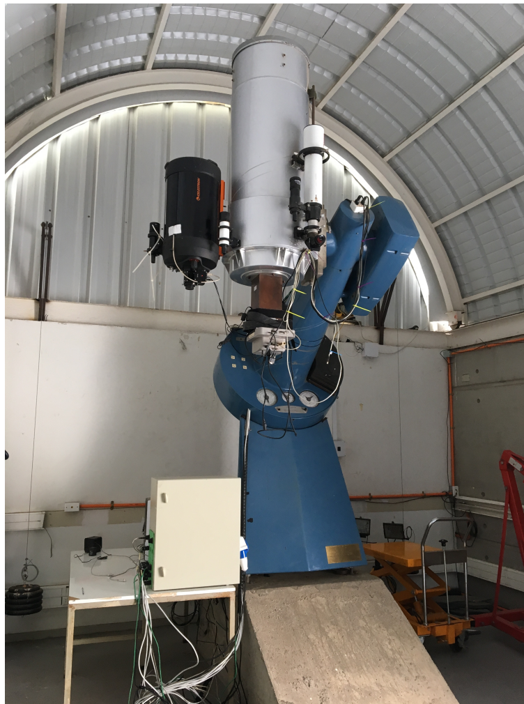
Figure 5.2.1: General view of the PUC40 telescope installed at Santa Martina's Golf Club. It is possible to appreciate the typical Boller & Chivens departed Hour Angle Axis.
