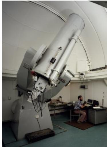
Figure 2.2.1: The Eso 50cm Fork equatorial design
