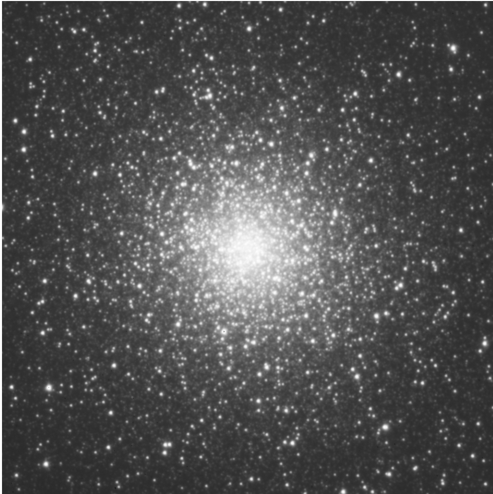
Figure 5.2.5: Integration of a 2h session on the NGC104 Globular cluster using the PUC40cm telescope imager. The result presented is the combined sum of 40 consecutive 180s exposures with a Johnson & Cousins R filter with no auto-guiding. The roundness of the images of stars shows that the system can perfectly handle 3mn exposures without the need of guiding, partially thanks to the effect of using the advanced pointing model described in Section 4.2.
