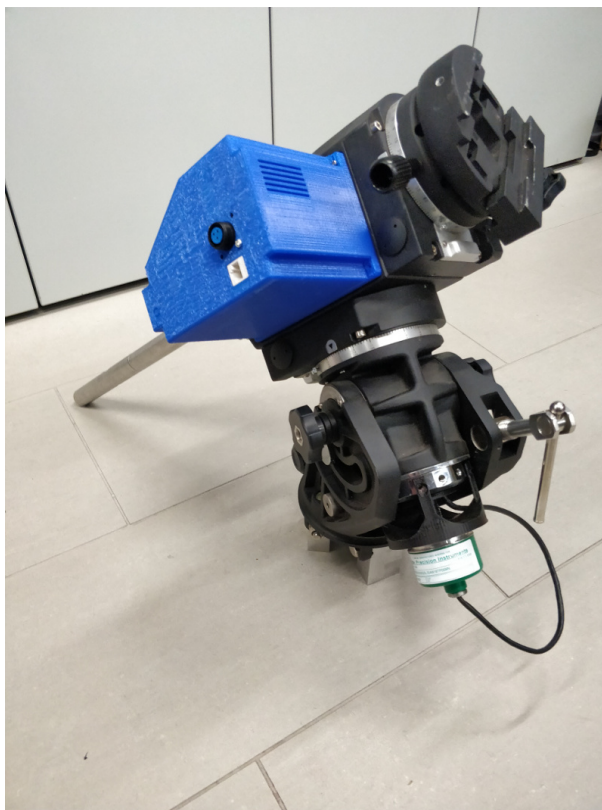
Figure 4.1.12: Picture of the setup and the encoder installation on the main axis of the commercial mount
