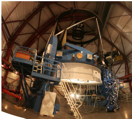
Figure 2.2.3: The Magellan Clay 6.5m AltAz telescope
