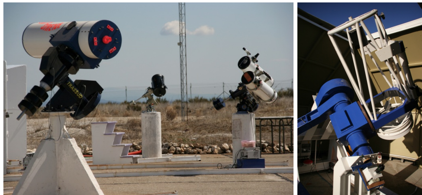
Figure 2.2.2: Telescopes on German and British Equatorial mounts
