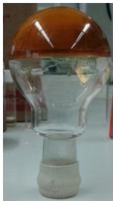
Figure 6.16. Gel formed with complex 60 and TEOS (molar ratio 1:30).
