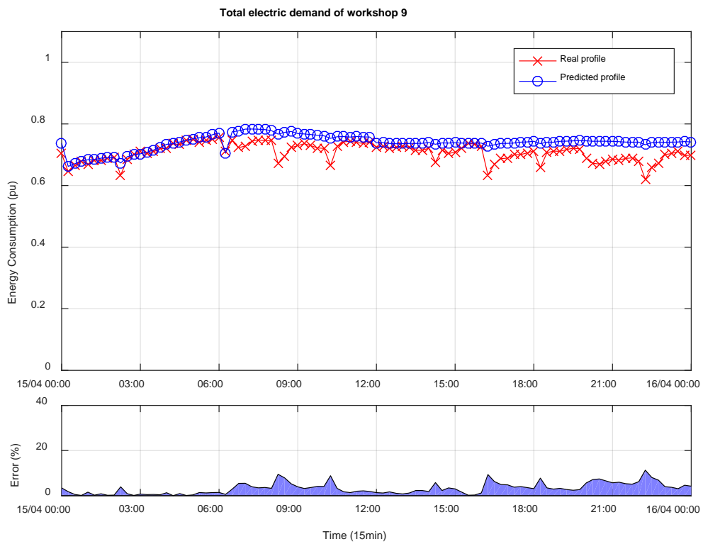
Figure A.21: Prediction result of the total electric demand of workshop 9: 15 th April 2015.
