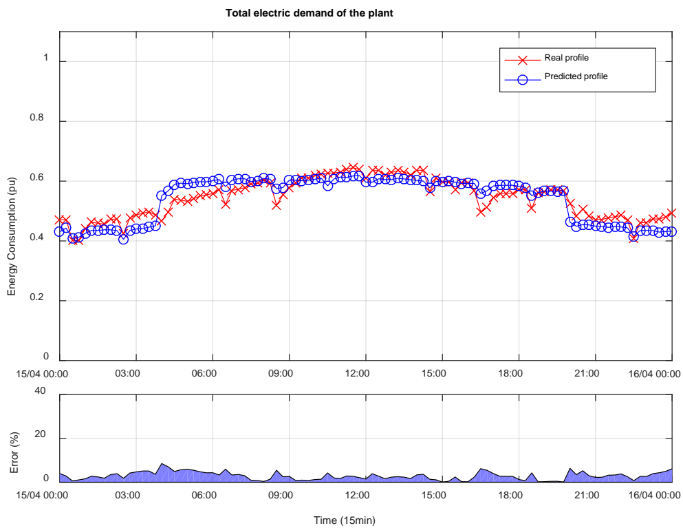
Figure A.3: Prediction result of the total electric demand of the plant: 15 th April 2015.
