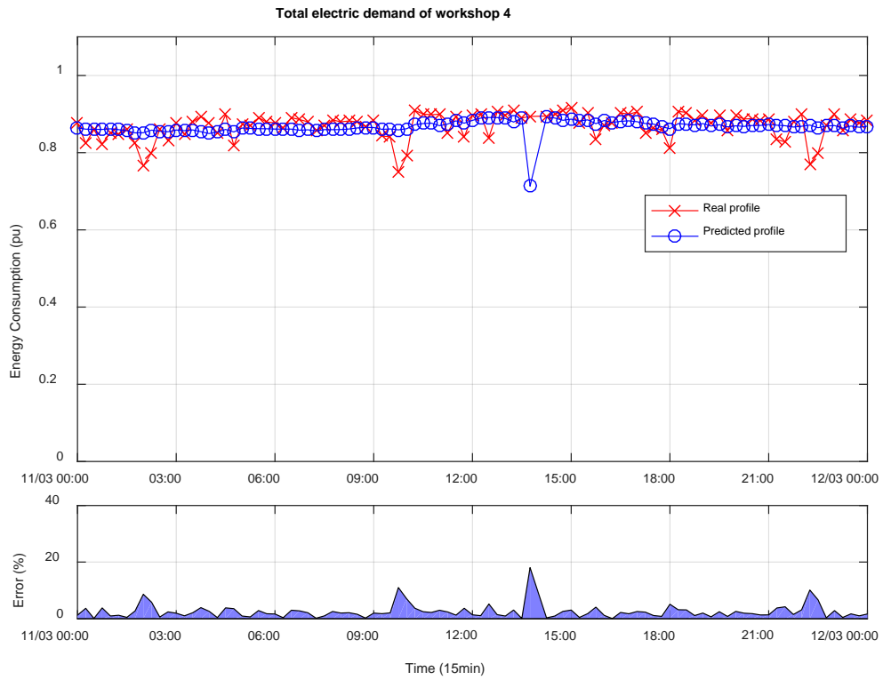
Figure A.14: Prediction result of the total electric demand of workshop 4: 11 th March 2015.
