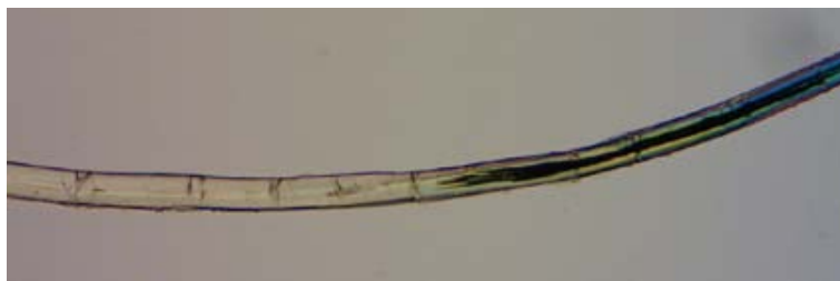
Figure 5. Hemp fibre from sample 24_v. The lumen is the same width as the fibre walls. Cross-marks tend to be more vertical. Original magnification was 200x.
