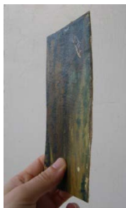
Figure 20. Piece of a painting ( 76 ), with a cotton canvas and DP 660. It is clear that in this case the paint layer is holding the canvas and not the other way around, since the untacked textile would not stay up right on its own.
