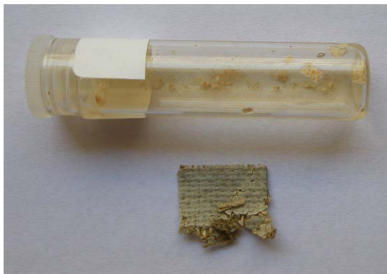
Figure 8. Vinegar test for sample 54 . This modern priming layer from the beginning of the 20 th C is clearly not dissolved by the acetic acid: primer particles can be seen inside the glass vial.
