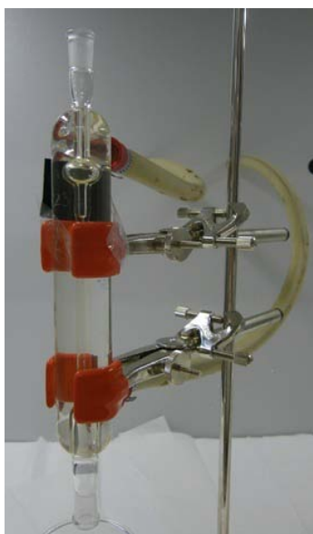
Figure 10. Glass viscometer used. Water kept at 25°C coming from the nearby water-bath is constantly circulating around the capillary tube where the measured is pulled up, so that its temperature is constant.
