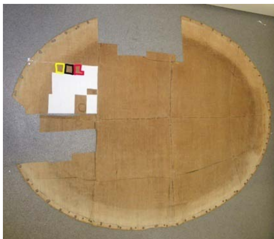
Figure 14. Locations where the sub-samples used for evaluation of sample cleaning procedures come from the old glue lining 112: MD-1 (red); MD-4 (black); MD-5 (yellow).
