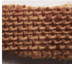
Figure 27. Sample 68: jute threads can be seen to run vertically, cotton threads run horizontally.
