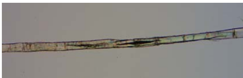
Figure 6. Ramie fibre from sample 18_v. The lumen varies in width along the fibre. Original magnification was 200x.
