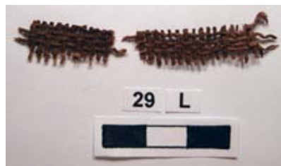
Figure 1. Mixed sample: the threads running vertically are jute, the ones running horizontally are cotton.
