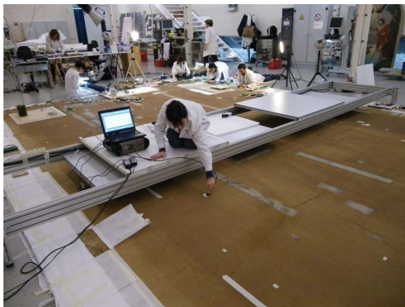
Figure 28. Taking NIR spectra from the reverse of the large painting El gran dia de Girona by Martí Alsina (MNAC 12084).
