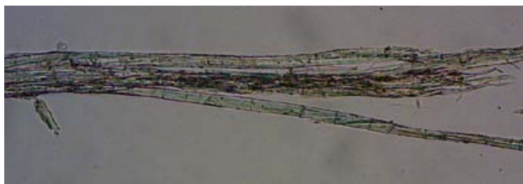
Figure 2. Fibres from sample 7_v. The textile is so degraded that identification on the basis of morphological features is difficult. Original magnification was 200x (All the images in this chapter were taken with a DinoEye® AM423X, a very handy new small camera that fits into the microscope in the place of the original eyepieces. Original magnification was thus 10x from the objective and 20x from the camera).
