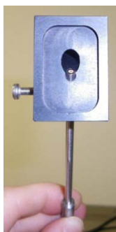
Figure 6. The purpose-made attachment to the probe to have the beam always at a 45° angle. The beam diameter is about 2 mm.
