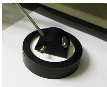
Figure 7. Optical light probe with the purpose made attachment on the white reference calibration pad where samples were measured.
