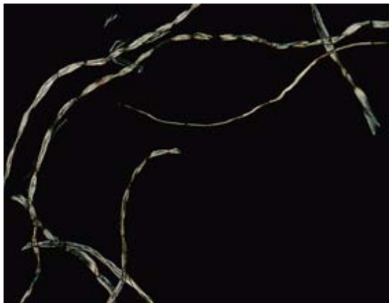
Figure 3. Sample 95_v, cotton observed with a dark field, convolutions are more easily seen. Original magnification was 100x.
