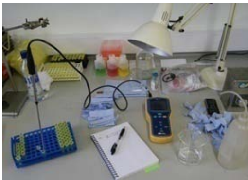
Figure 10. Set-up for pH measurement of the prepared samples. Note that the ISFET electrode can be left inside the plastic vial during pH measurement as it stands on its own.
