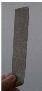
Figure 21. Animal glue applied to bare canvas. The glue makes the canvas already rigid enough to be kept upright.
