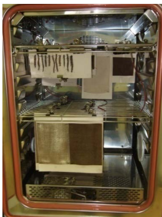
Figure 5. The samples inside the climate chamber running at 90°C and 65% RH
