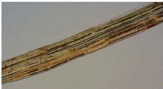
Figure 7. Jute fibres from sample 68_v. Fibres are all stuck together and the broken lumen can be clearly seen. Original magnification was 200x.
