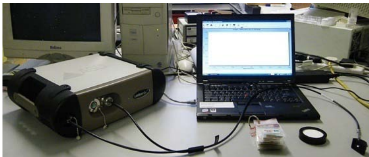
Figure 5. Labspec 5000 (Analytical Spectral Devices, USA). The instrument, the fibre optics probe, the computer and the white reference calibration pad.
