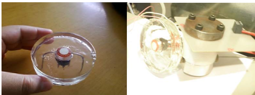
(a) (b) Figure 1: (a) Picture of the TGS embedded inside the sensing chamber with metallic inlet and outlet connections (b) picture of the concentrator chamber connected with the TGS.
