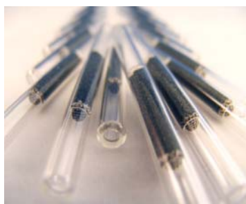
Figure 2: Commercial thermal desorption preconcentration tube from CAMSCO inc., used with permission [31]
