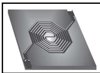
Figure 10: Schematic view of the fabricated spiral micro-concentrator [81]
