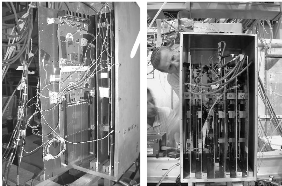
Figure 6.6 The CMS tracker used as a reference telescope triggered by the pair of edgeless diodes, which consists of six planes with vertical microstrip silicon detector modules (TOBs) cooled to -20\text{ }^{\circ}\text{C} .
