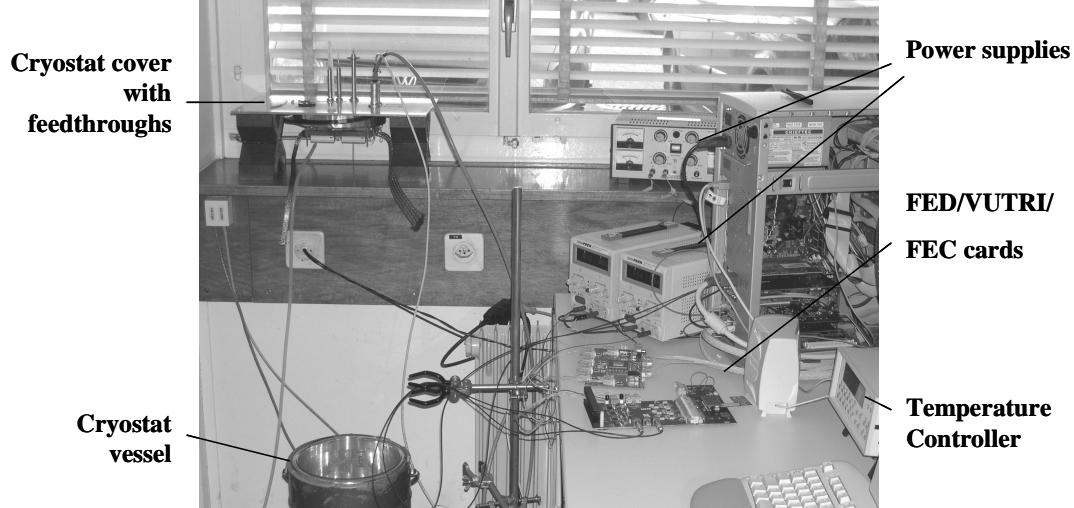
Figure 5.7 Experimental setup for low temperature readout electronics tests.
