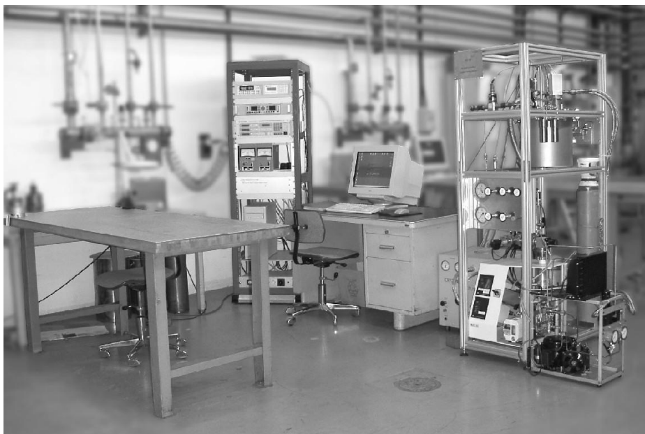
Figure 4.1 Experimental setup for heat transfer measurements in microtubes at cryogenic temperatures sitting at the Low Temperature Laboratory at CERN [27].
