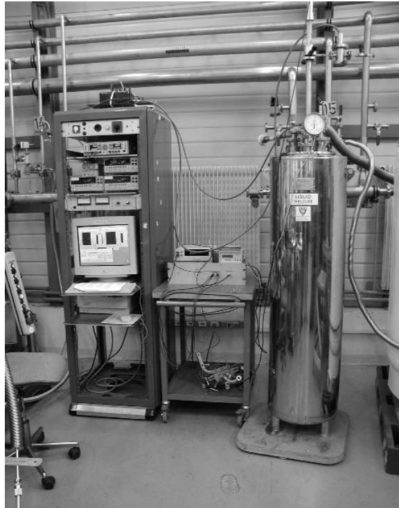
Figure 3.2 Experimental setup to measure the thermal dilatation of fused quartz filled epoxies, sitting at the Low Temperature Laboratory at CERN.
