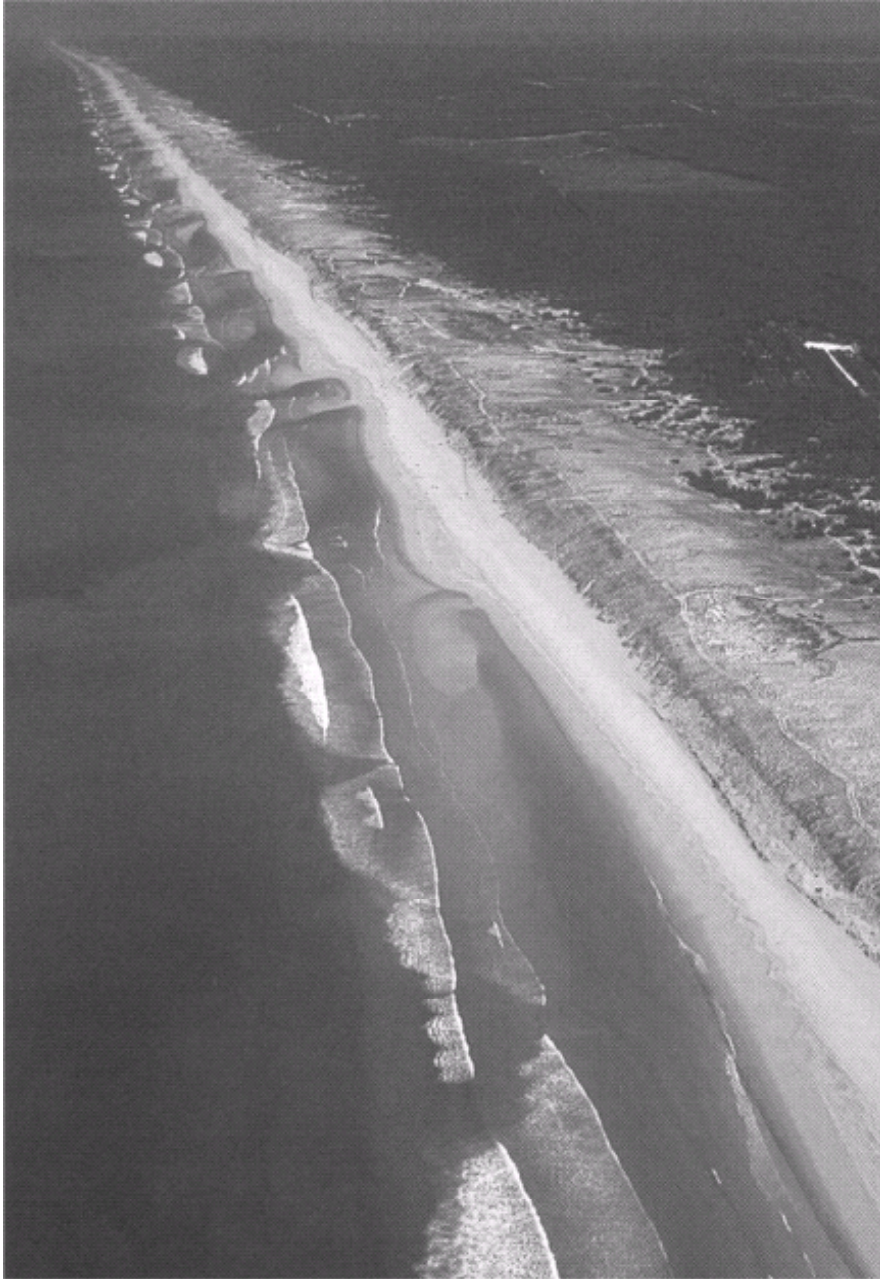
Figure 1.2.9: Photography of the Southern part of the French Atlantic coast (Les Landes). A system of rhythmic oblique sand bars with a wave length of some 400 meters is often observed in this environment. The bars usually migrate southward with a daily average celerity of about 2.5m/day (see Lafon et al. (2002))
