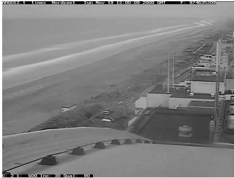
Figure 1.2.1: Oblique time exposure image of two shore-parallel sand bars in the surf zone of the Noordwijk beach, in The Netherlands, on 19 th November 2000. Wave breaking over two submerged shore-parallel sand bars produces white foam that appears as two white bands in this 10-minute time exposure image.
