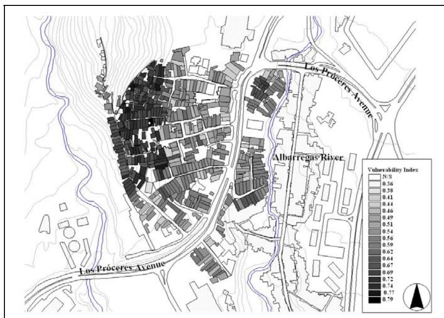
Map 6.14: New vulnerability index distribution in La Milagrosa Barrio, considering the adjacency parameter (N/S: Not studied).
