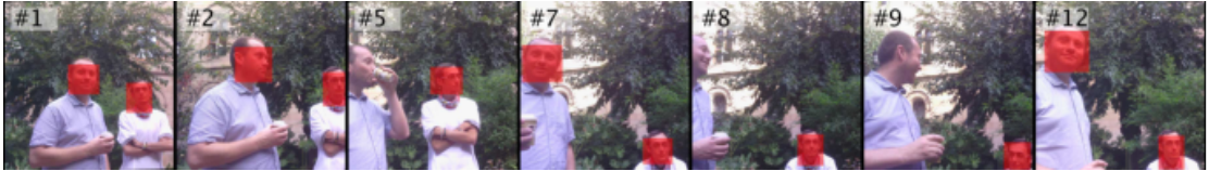
Figure 3.1: Detected faces (seeds) are shown by red bounding boxes in a sequence. An example of false negatives can be observed in frames 8 and 9. Only a sub-sample of the original sequence is shown.
