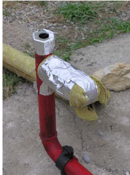
Figure 2.6. Pressure measurement equipment (electronic pressure transmitter) located 0.05 m upstream the outlet orifice and temperature measurement equipment at the nozzle jet exit (uncoated K-type thermocouple (nickel-chromium/nickel-aluminium)).
