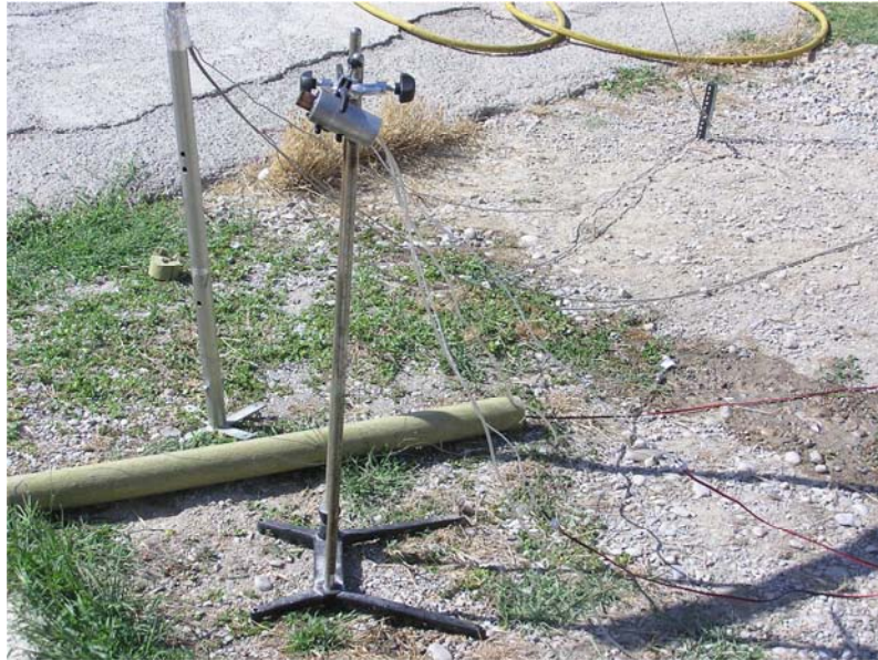
Figure. 2.10. Heat flux sensor: heat flux transducer and radiometer 64-20T-20R(S)-20898 model, with a water cooling system.
