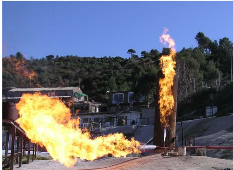
Figure 1.9. Two phase propane jet fires, obtained from vertical and horizontal releases.
