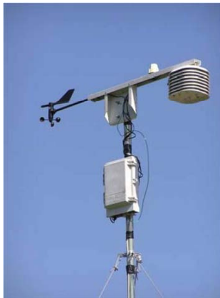
Figure 2.12. A view of the meteorological weather station (Davis Instruments, GroWeather).
