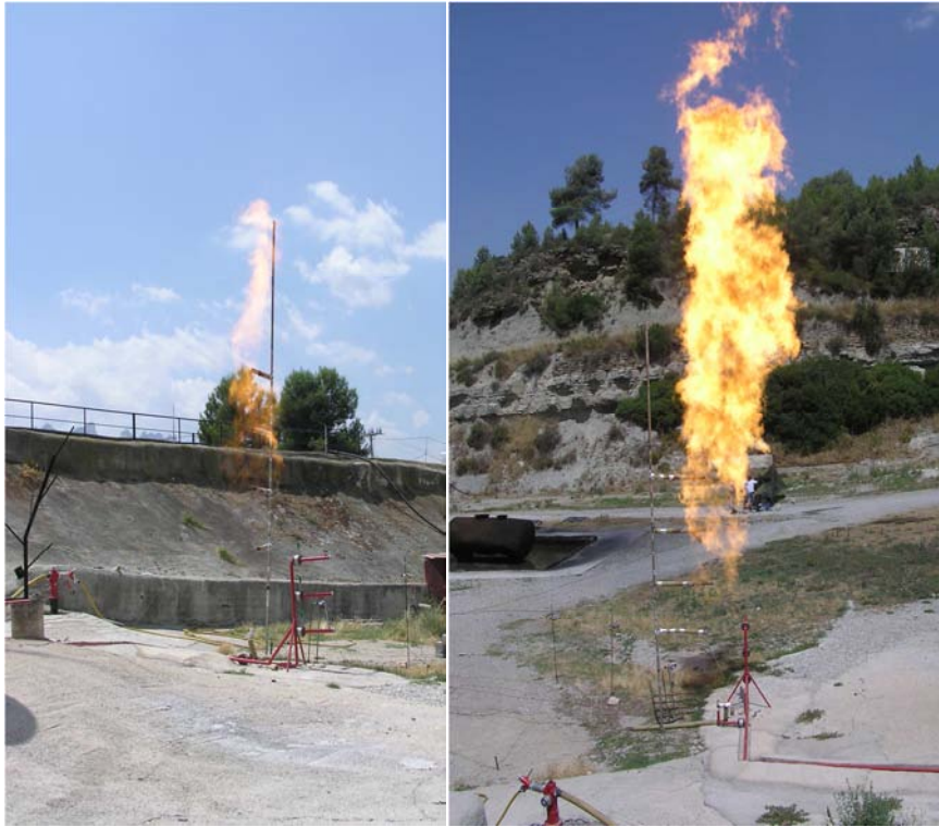
Figure 5.1. Visible images of vertical jet flames of propane obtained with gas phase and d = 20 mm (left), and two-phase flow and d = 43.1 mm (right).
