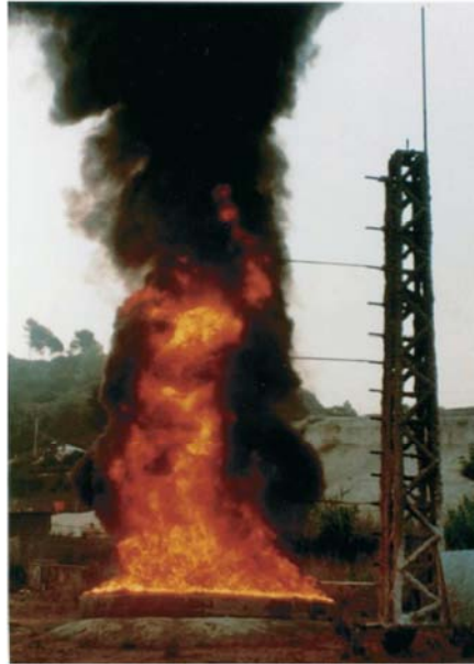
Figure 1.7. An outdoor pool fire. Pool diameter: 4 m; fuel: gasoline (taken from Chatris et al. , 2001).
