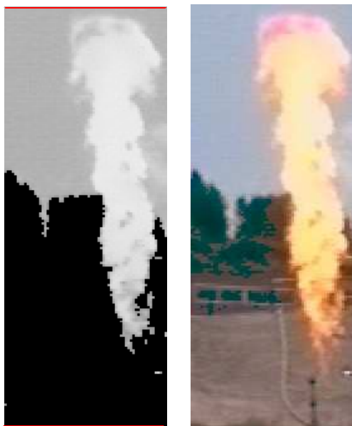
Figure 3.5. Visible image (Fig. 3.3) (right) and using a lower value for the intensity of colour: the flame tip is not detected (left).
