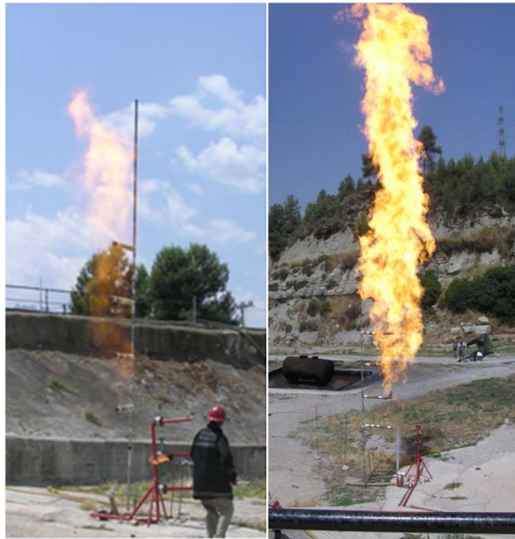
Figure 2.16. Visible images of vertical jet flames of propane obtained with: gas phase and d = 12.75 mm (left); two-phase flow and d = 43.1 mm (right).
