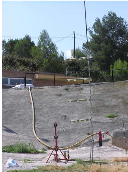
Figure 2.8. The temperature measurement equipment: a set of three thermocouples B-type and one S-type measuring the temperature distribution on the jet flame axis.
