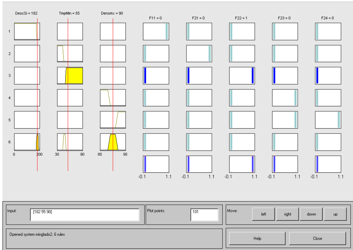
Figure 8.12. Fuzzy reasoning when Fault "Excess of steam to the refinery" has been simulated.
