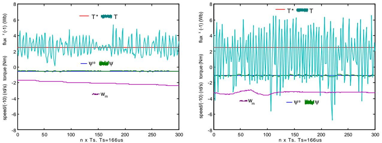
Figure 5.23. Stator flux, torque and speed motor\_1.5kW responses in Fuzzy Logic DTC (left) and classical DTC (right). Load resistance is  $8\Omega$ . Torque reference value is 2.45Nm, i.e.  $T=25\%T_n$ .
