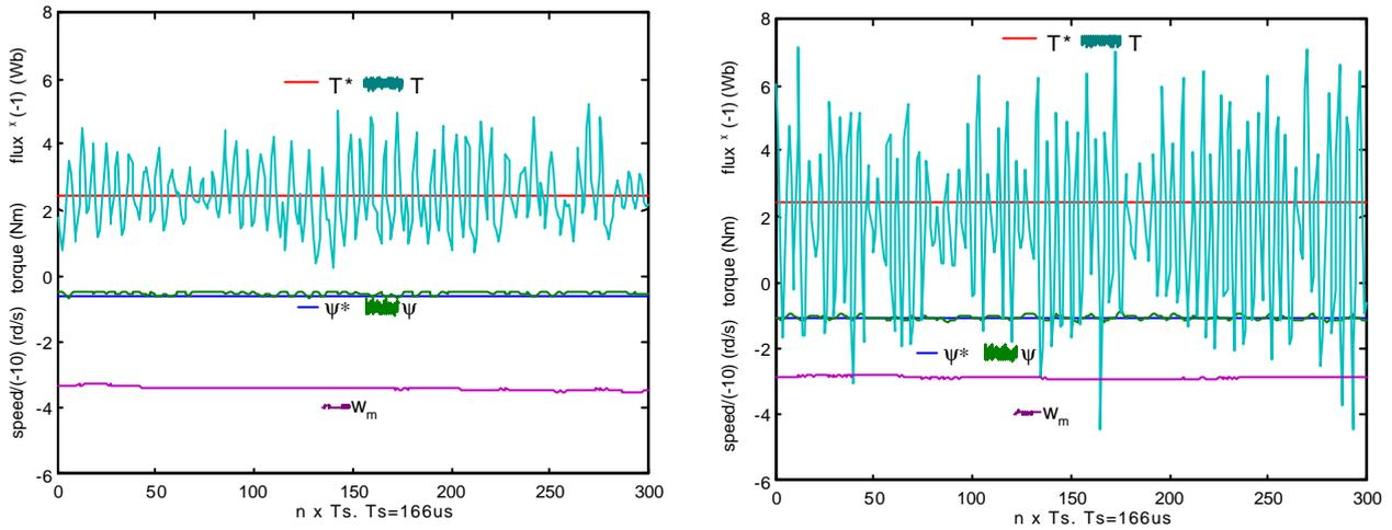
Figure 5.22. Stator flux, torque and speed motor\_1.5kW responses in Fuzzy Logic DTC (left) and classical DTC (right). Load resistance is  $4\Omega$ . Torque reference value is 2.45Nm, i.e.  $T=25\%T_n$ .
