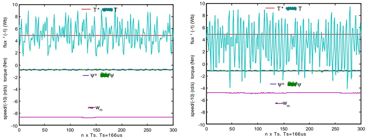
Figure 5.20. Stator flux, torque and speed motor\_1.5kW responses in Fuzzy Logic DTC (left) and classical DTC (right). Load resistance is  $4\Omega$ . Torque reference value is  $4.9\text{Nm}$ , i.e.  $T=50\%T_n$ .
