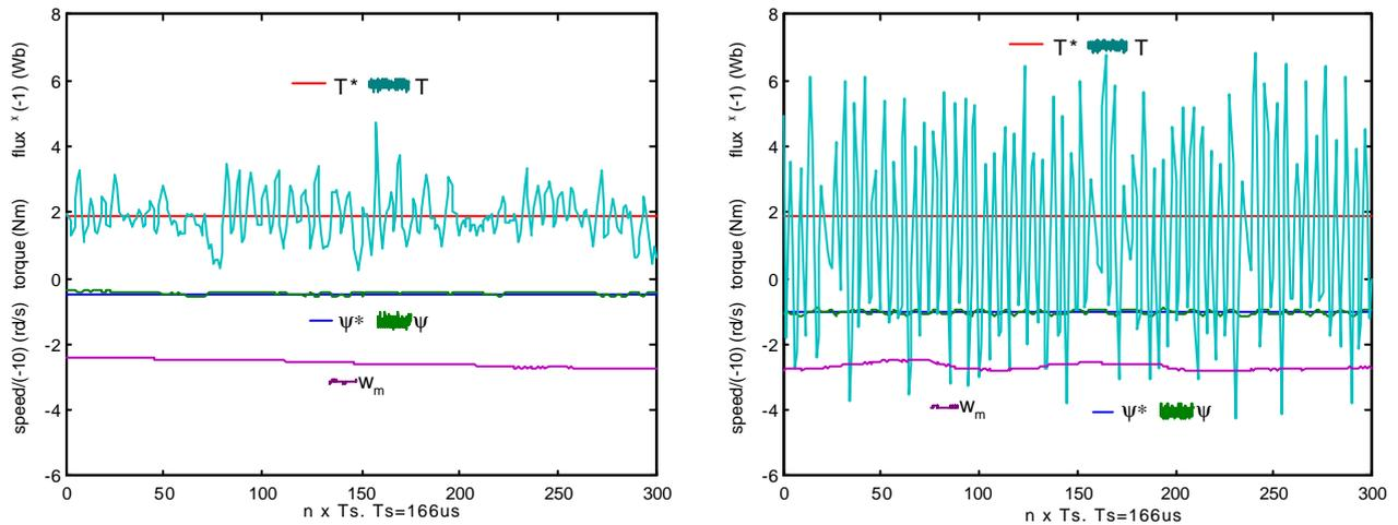
Figure 5.25. Stator flux, torque and speed motor\_1.5kW responses in Fuzzy Logic DTC (left) and classical DTC (right). Load resistance is  $8\Omega$ . Torque reference value is 1.9Nm, i.e.  $T=19\%T_n$ .
