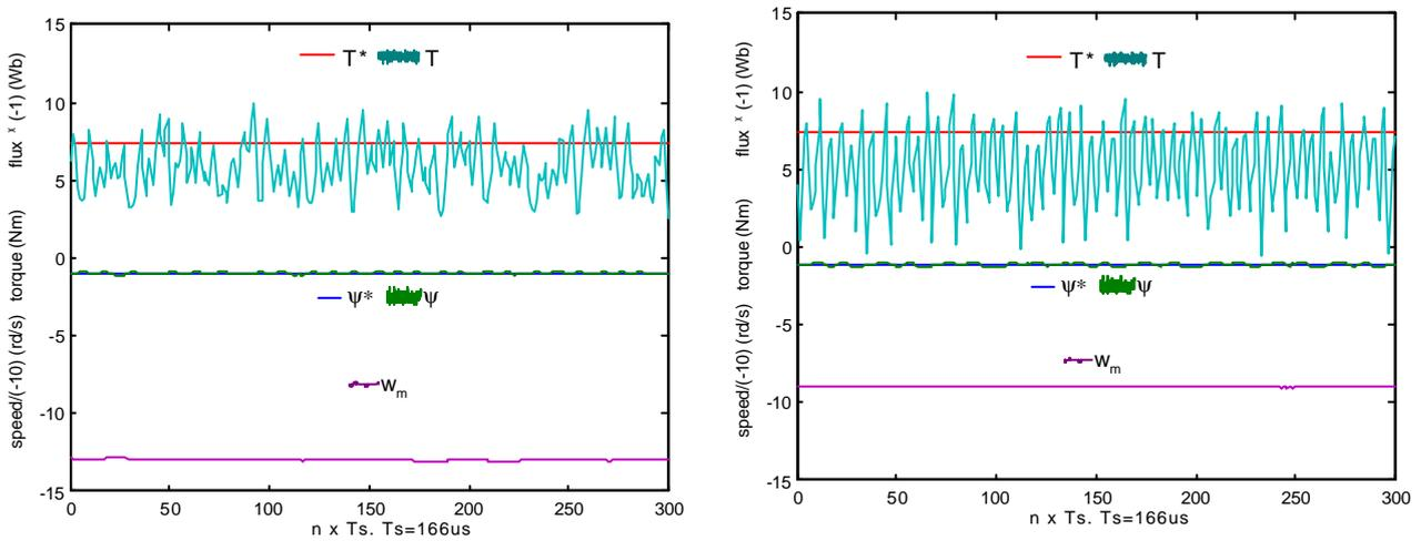
Figure 5.19. Stator flux, torque and speed motor\_1.5kW responses in Fuzzy Logic DTC (left) and classical DTC (right). Load resistance is  $8\Omega$ . Torque reference value is  $9.8\text{Nm}$ , i.e.  $T=75\%T_n$ .
