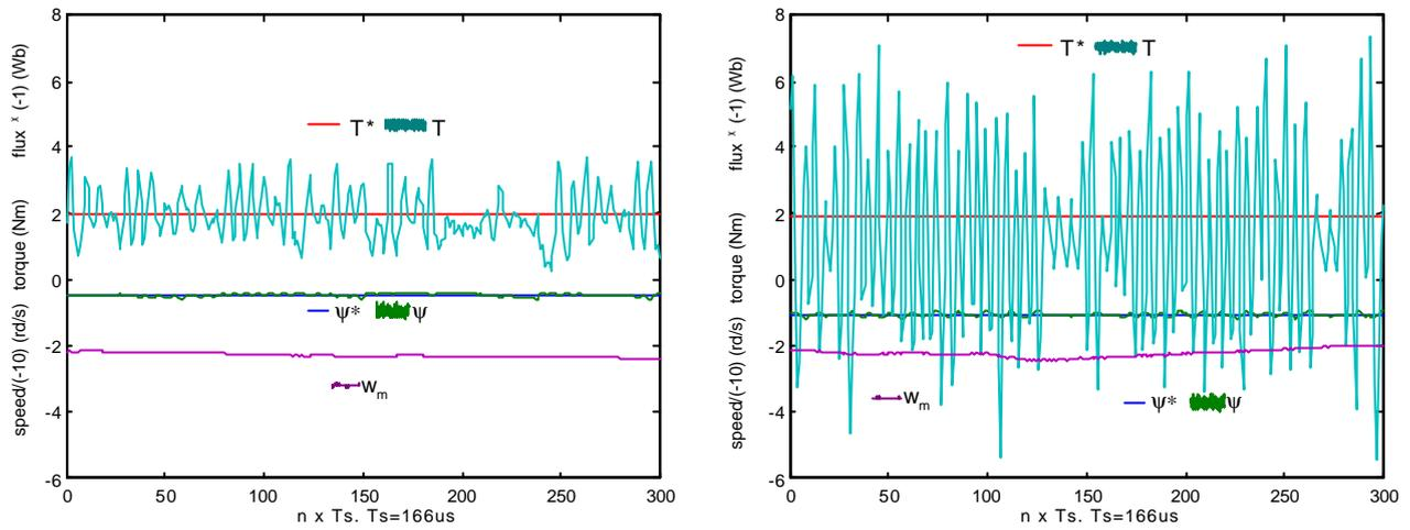
Figure 5.24. Stator flux, torque and speed motor\_1.5kW responses in Fuzzy Logic DTC (left) and classical DTC (right). Load resistance is  $4\Omega$ . Torque reference value is 1.9Nm, i.e.  $T=19\%T_n$ .
