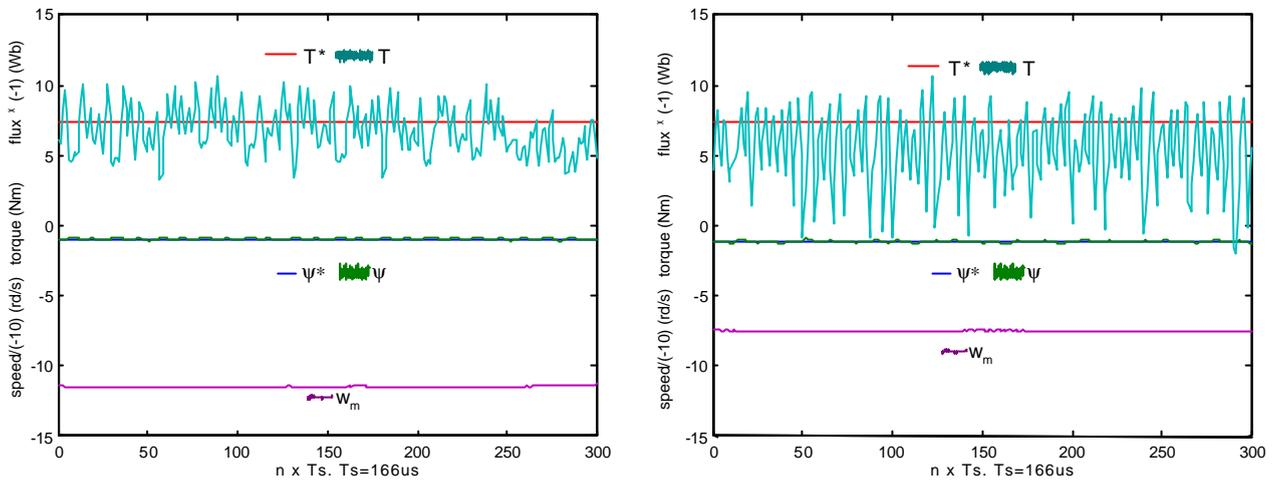
Figure 5.18. Stator flux, torque and speed motor\_1.5kW responses in Fuzzy Logic DTC (left) and classical DTC (right). Load resistance is  $4\Omega$ . Torque reference value is  $7.35\text{Nm}$ , i.e.  $T=75\%T_n$ .
