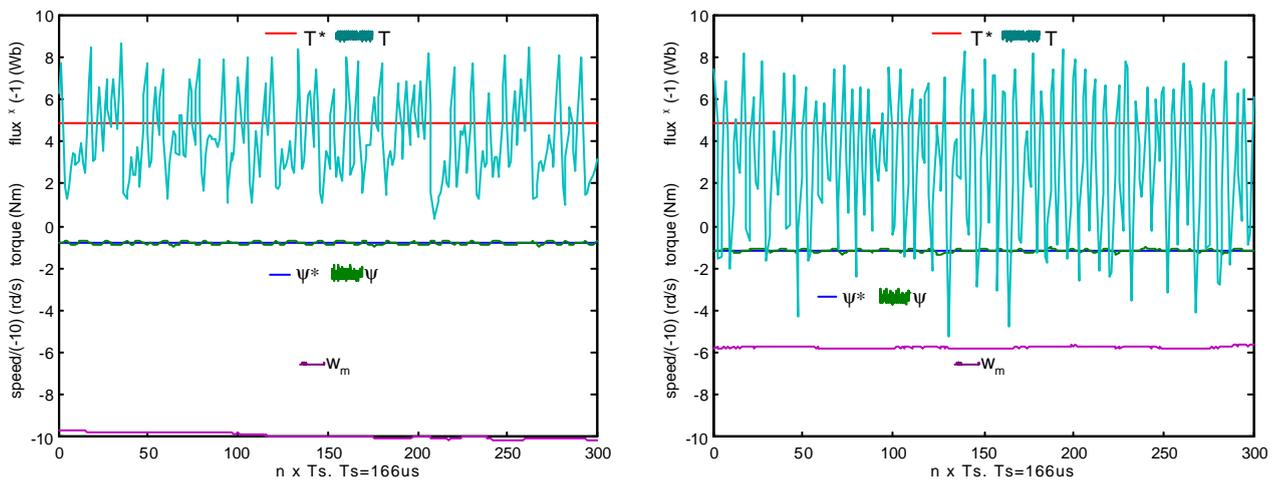
Figure 5.21. Stator flux, torque and speed motor\_1.5kW responses in Fuzzy Logic DTC (left) and classical DTC (right). Load resistance is  $8\Omega$ . Torque reference value is  $4.9\text{Nm}$ , i.e.  $T=50\%T_n$ .
