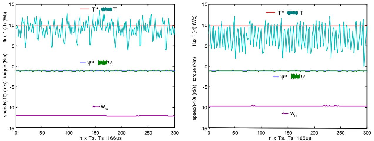
Figure 5.16. Stator flux, torque and speed motor\_1.5kW responses in Fuzzy Logic DTC (left) and classical DTC (right).
