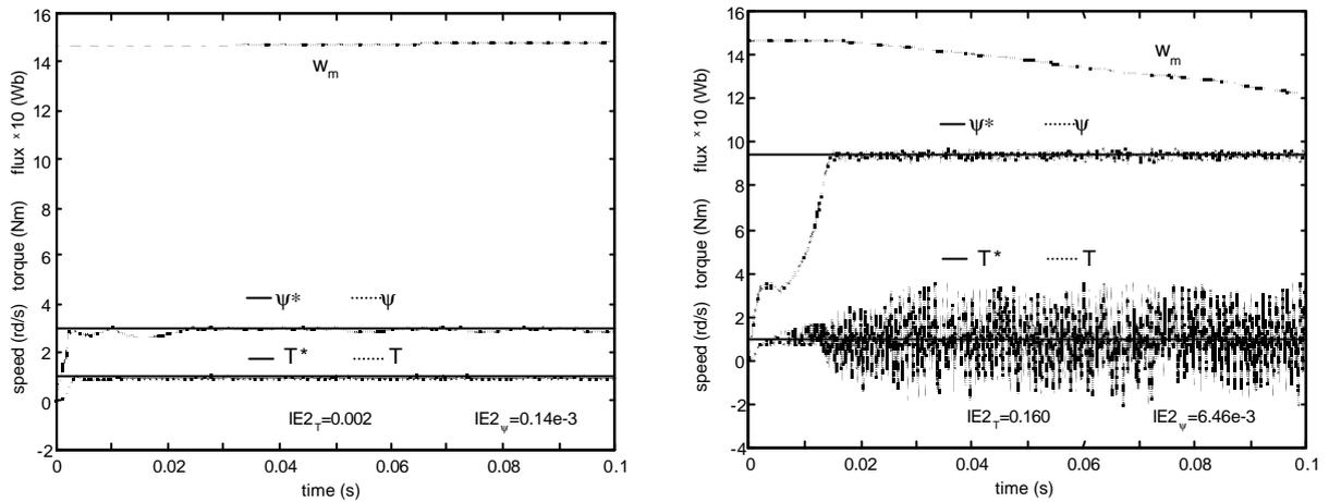
Figure 3.14 A. Stator flux, torque and speed motor\_1.5kW responses in Fuzzy Logic DTC (left) and classical DTC (right).  $T=10\%T_n$ ,  $w_m=10\%w_{nm}$ . Notice the IE2 flux and torque error indexes values.
