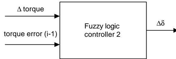
Figure 3.8. Fuzzy logic controller increment\_duty ratio estimator.
