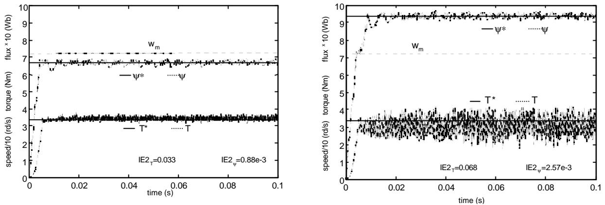
Figure 3.16 B. Stator flux, torque and speed motor\_1kW responses in Fuzzy Logic DTC (left) and classical DTC (right).  $T=50\%T_n$ .  $w_m=50\%w_{m1}$ . Notice the IE2 flux and torque error indexes values.
