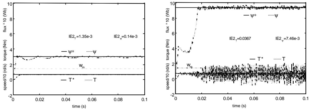
Figure 3.14 B. Stator flux, torque and speed motor\_1kW responses in Fuzzy Logic DTC (left) and classical DTC (right).  $T=10\%T_n$ ,  $w_m=10\%w_{nm}$ . Notice the IE2 flux and torque error indexes values.
