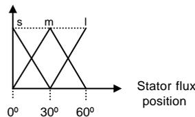
Figure 3.3. Stator flux position membership input.
