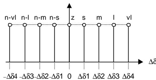
Figure 3.10. Increment duty ratio membership.
