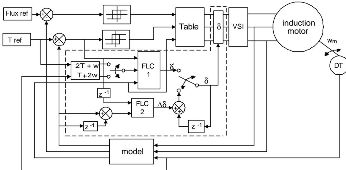
Figure 3.11. Schematic of the Fuzzy Logic DTC. In dashed line is separated the novel fuzzy controller part.
