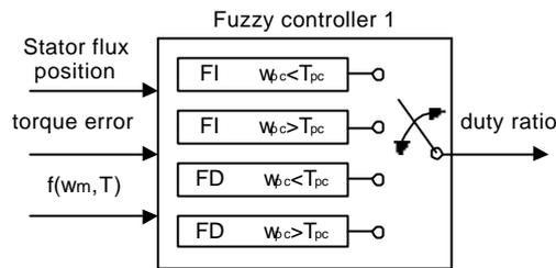
Figure 3.2. Fuzzy logic duty ratio estimator. It can be seen its four different groups of rules. Just one group of rules is used per iteration.
