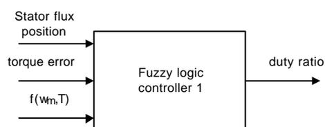
Figure 3.1. Fuzzy Logic duty ratio estimator
