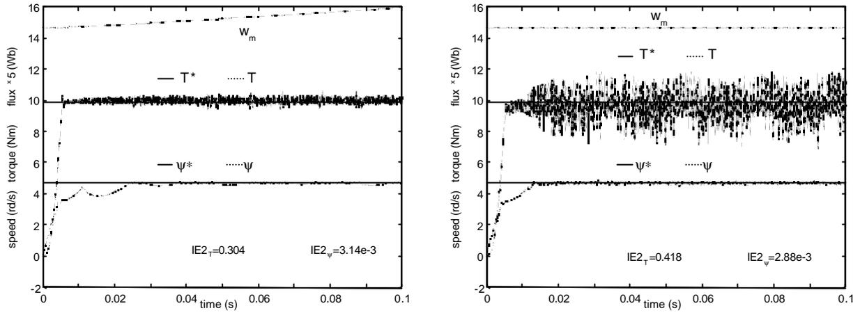
Figure 3.15 A. Stator flux, torque and speed motor\_1.5kW responses in Fuzzy Logic DTC (left) and classical DTC (right).  $T=100\%T_n$ ,  $w_m=10\%w_{nm}$ . Notice the IE2 flux and torque error indexes values.
