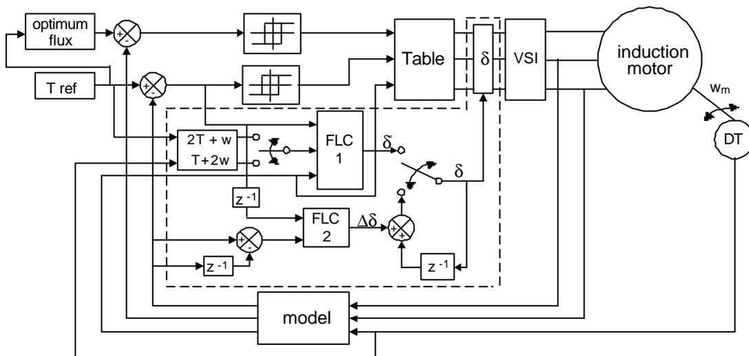
Figure 3.12. Flux reference optimised controller in a Fuzzy Logic DTC.
