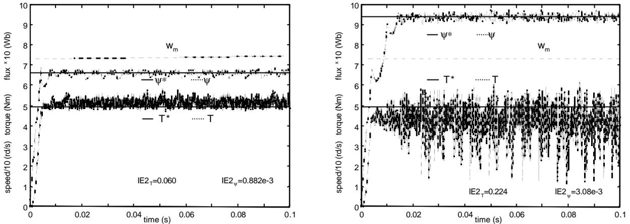
Figure 3.16 A. Stator flux, torque and speed motor\_1.5kW responses in Fuzzy Logic DTC (left) and classical DTC (right).  $T=50\%T_n$ .  $w_m=50\%w_{m1}$ . Notice the IE2 flux and torque error indexes values.
