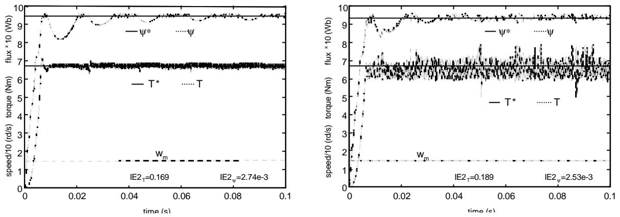
Figure 3.15 B. Stator flux, torque and speed motor\_1kW responses in Fuzzy Logic DTC (left) and classical DTC (right).  $T=100\%T_n$ ,  $w_m=10\%w_{nm}$ . Notice the IE2 flux and torque error indexes values.
