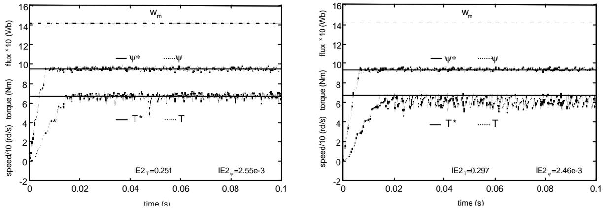
Figure 3.13 B. Stator flux, torque and speed motor\_1kW responses in Fuzzy Logic DTC (left) and classical DTC (right).  $T=100\%T_n$ .  $w_m=100\%w_{m}$ . Notice the IE2 flux and torque error indexes values.
