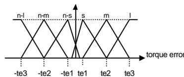
Figure 3.4. Torque error membership input.
