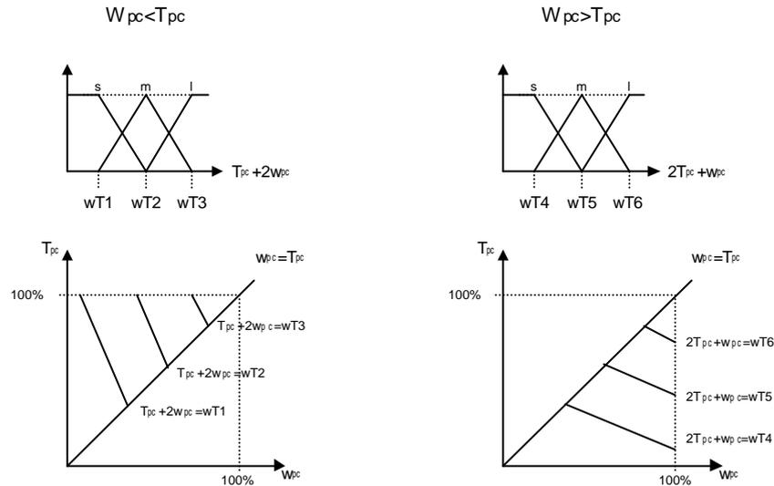
Figure 3.5. Working point membership inputs and the three different zones in the  $T, w$  plane. Left  $w_{pc} < T_{pc}$ . Right  $w_{pc} > T_{pc}$ .
