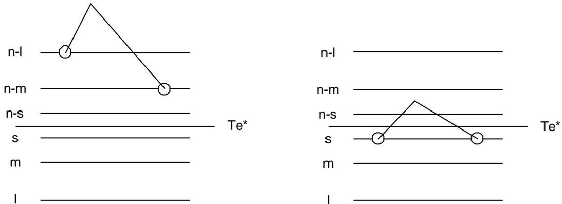
Figure 3.7. It can be seen the evolution of the torque during one  $T_z$ . Left: if the torque increment is negative medium, and the error in the previous iteration was negative large, the duty ratio increment has to be small. This case corresponds to the second rule (see section A.2.2). Right: if the torque increment is zero, and the error in the previous state was small, the increment in duty ratio has to be zero. This case corresponds to the seventeenth rule (see section A.2.2).
