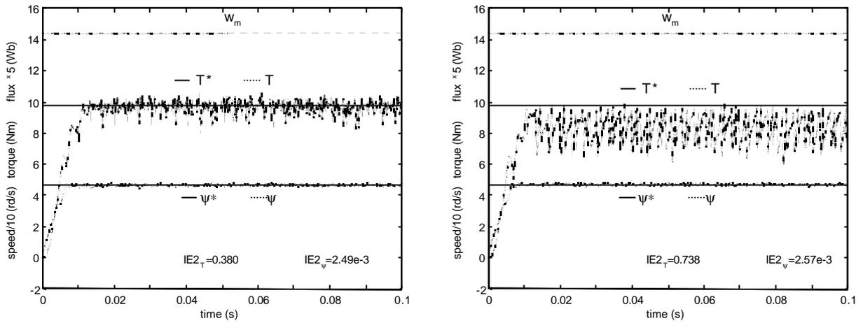
Figure 3.13 A. Stator flux, torque and speed motor\_1.5kW responses in Fuzzy Logic DTC (left) and classical DTC (right).  $T=100\%T_n$ .  $w_m=100\%w_{m}$ . Notice the IE2 flux and torque error indexes values.
