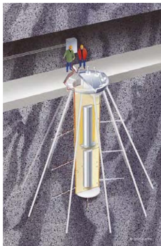
Figure 6.2. Principle design of the Temperature Buffer Test (SKB, 2005).
