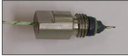
Figure 4.19: Temperature sensor (thermocouple type K with weld point).
