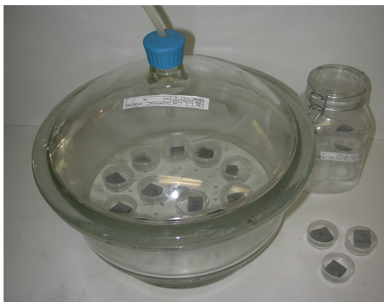
Figure 3.4: Specimens and containers used to evaluate the water retention curve.
