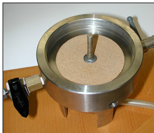
Figure 4.23: Bottom lid with the heater already installed.
