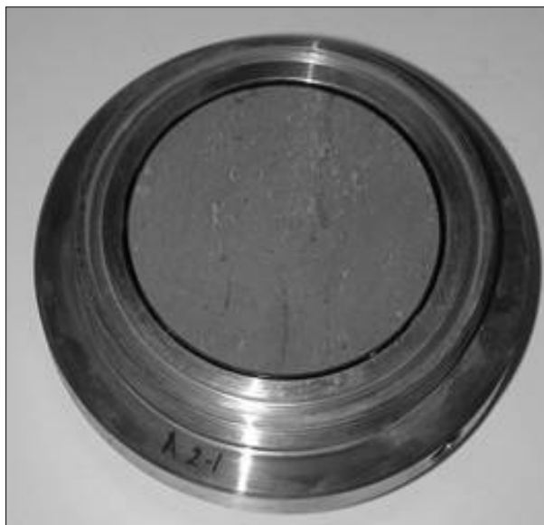
Figure 3.15: Sample pasted to the ring by means of epoxy resin
