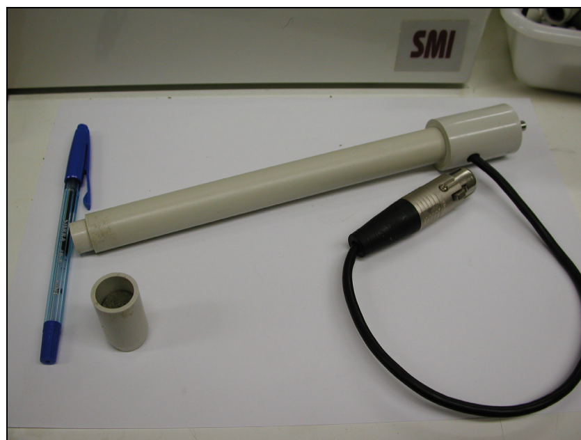
Figure 3.2: Transistor psychrometer sensor (Soil Mechanics Instrumentation, SMI) used to measure the total suction in Opalinus clay rock (Dimos, (1991)).
