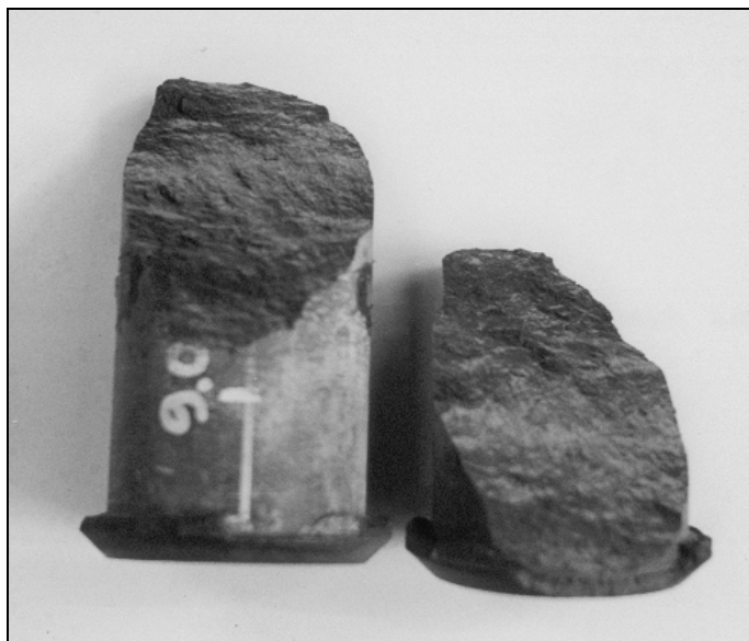
Figure 3.37: Sample C3 after the failure. Sample C3 presents the stratification planes inclined between 65^\circ and 70^\circ with respect to the longitudinal axis. Failure occurs in a plane inclined between 40^\circ and 43^\circ with respect to the longitudinal axis.
