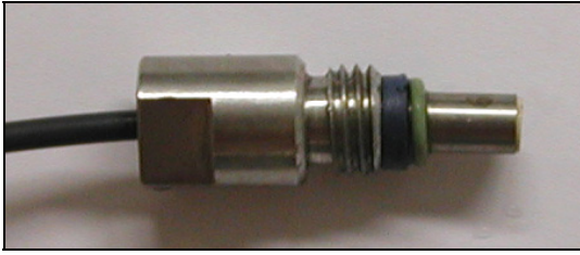
Figure 4.18: Miniature pore water pressure sensors (DRUC, model PDCR 81).
