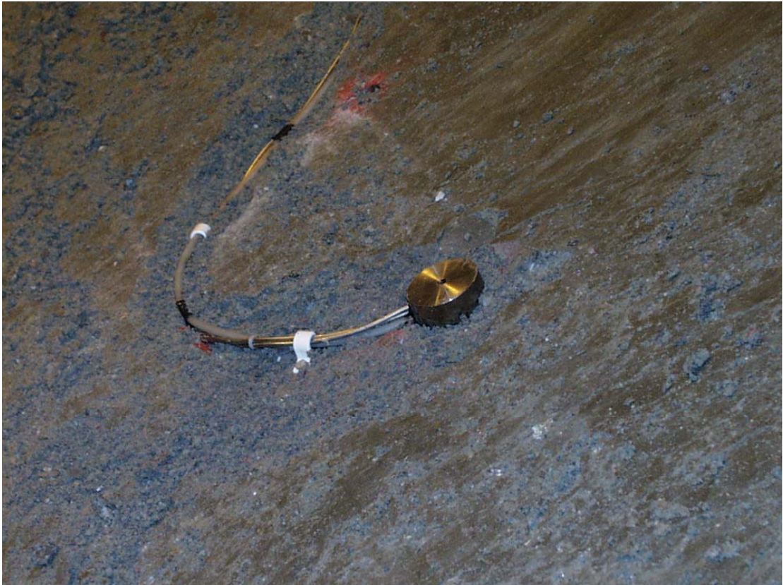
Figure 4.45: Detail of a DPPS placed perpendicularly to the layer (AITEMIN, 1999).
