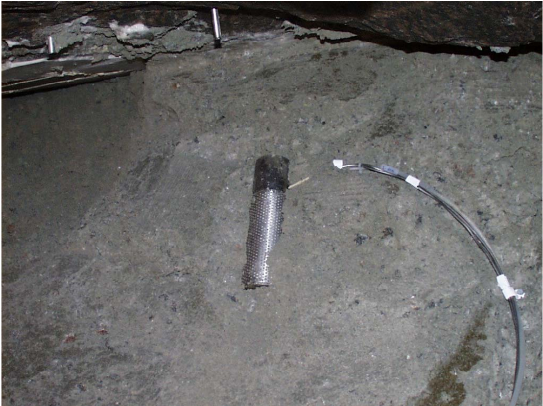
Figure 4.46: Detail of a DPPS placed in parallel with the layer (AITEMIN, 1999).
