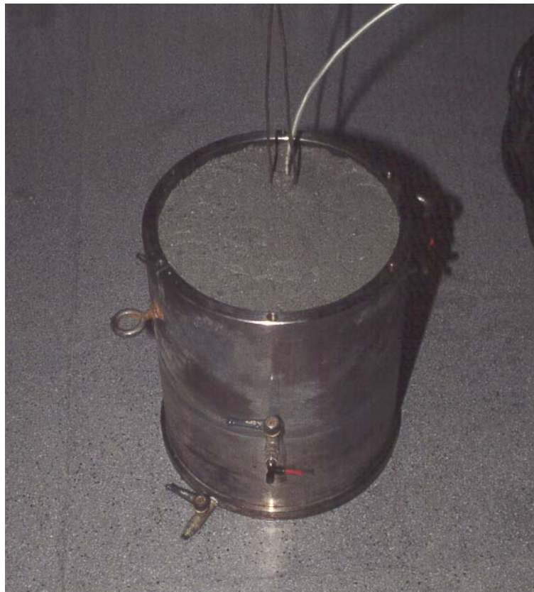
Figure 4.7: Compacted backfill specimen into the cell. Two stainless steel tubes (incoming and outgoing water from the DPPS) and a cable with the electric connexions came out from the backfill. A porous filter was placed at the top of the specimen and then the cell was closed.
