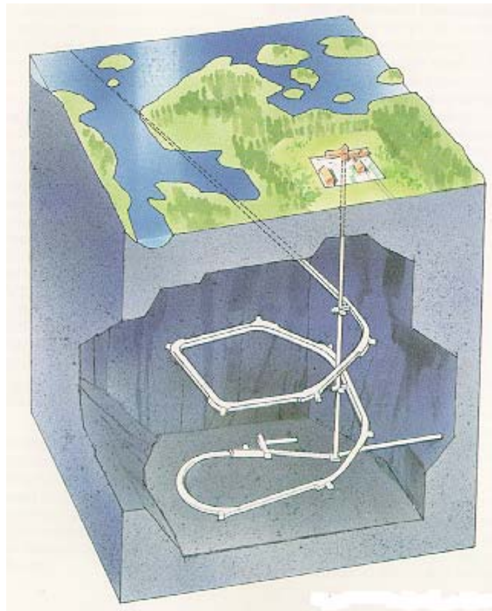
Figure 2.3: Schematic final layout of the Äspö Hard Rock Laboratory. Different experiments are being carried out in different tunnels (SKB, 1997).
