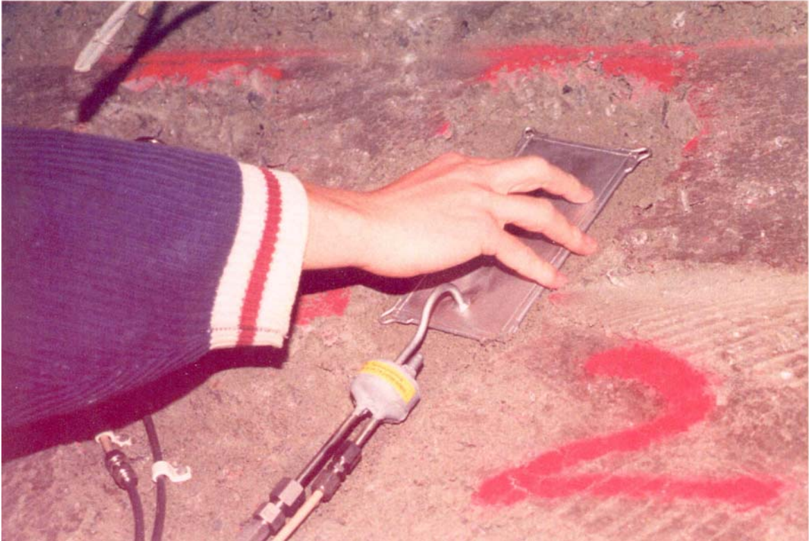
Figure 2.23: Glötzl total pressure cell placed in situ at one of the layers of backfill in the ZEDEX gallery (Gunnarsson et al. 2001).
