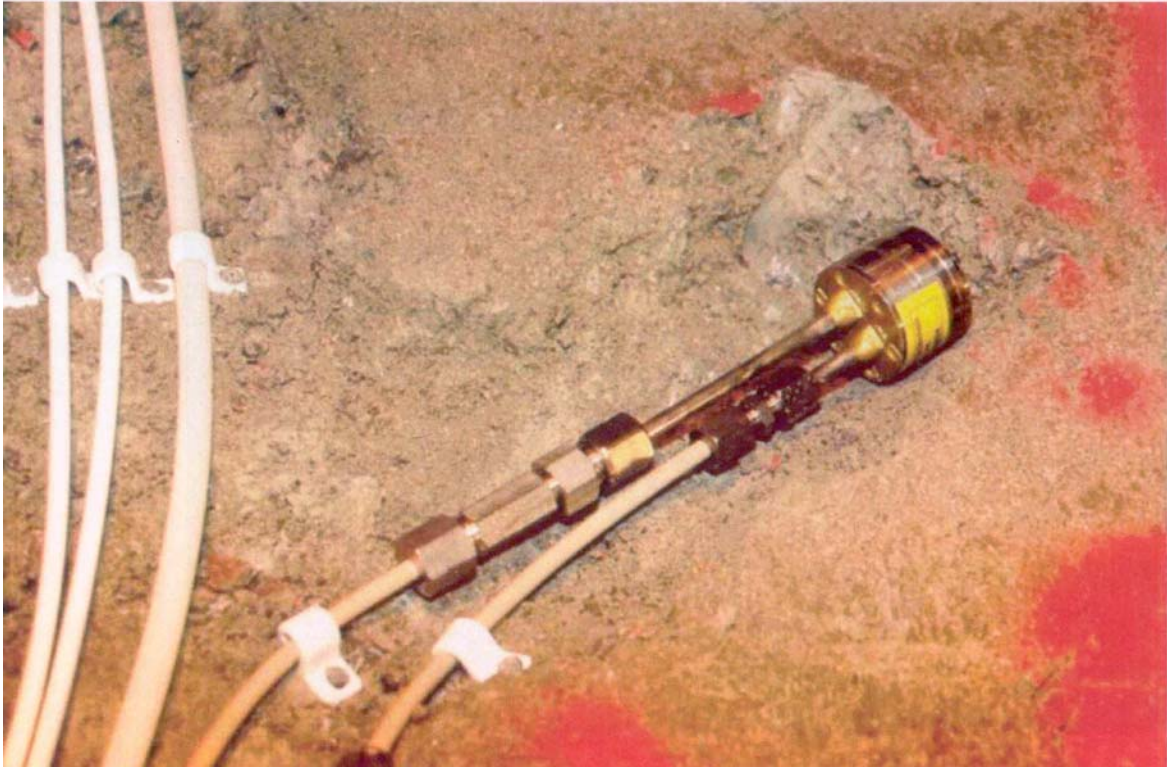
Figure 2.24: Glötzl pore water pressure cell placed in situ at one of the layers of backfill in the ZEDEX gallery (Gunnarsson et al. 2001).
