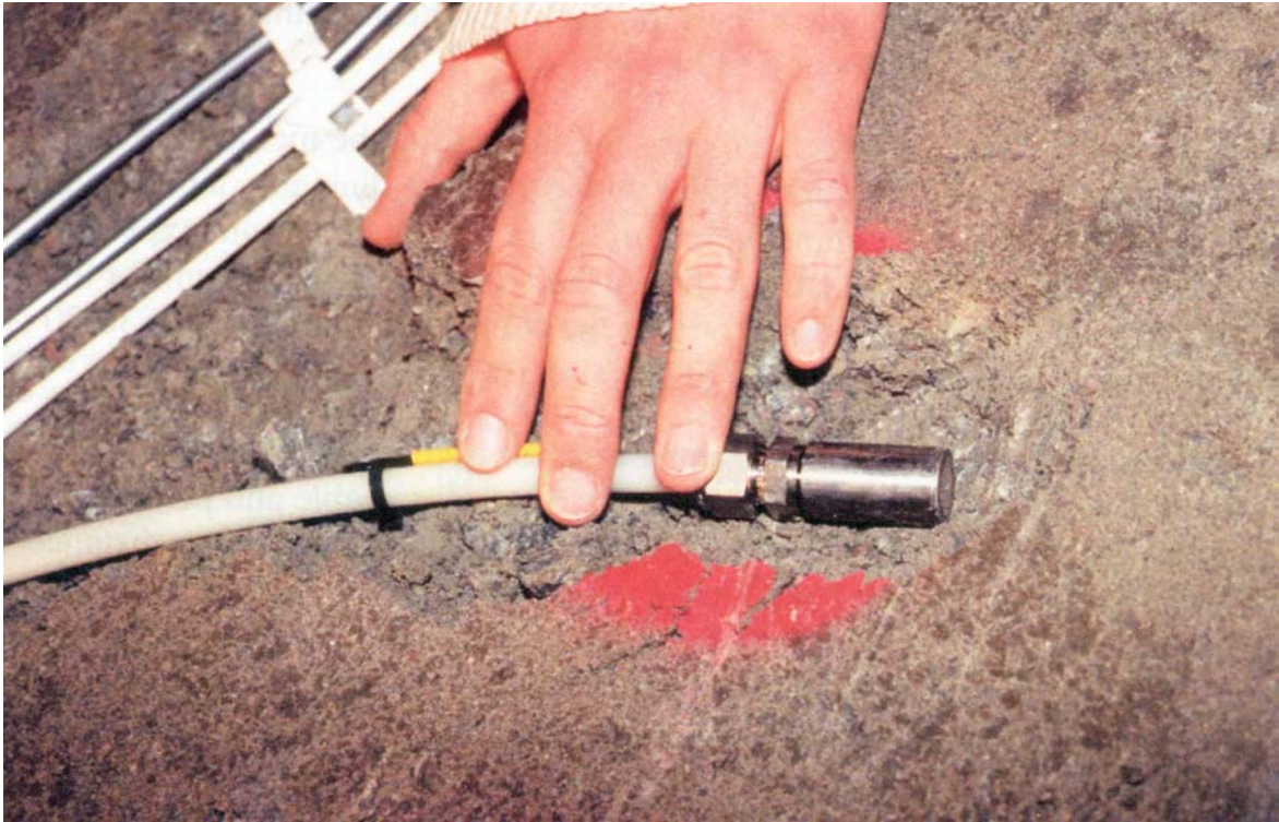
Figure 2.22: Wescor PST-55 placed in situ at one of the layers at the ZEDEX gallery (Gunnarsson et al. 2001). It can be observed that is very close to the surface of the layer.
