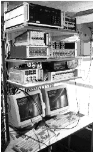
Figure D.3 Computer equipment to control the motion of the shaking-table
