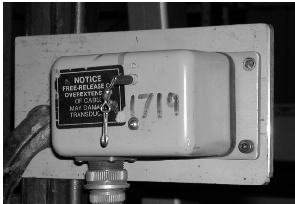
(a) Displacement transducer 'Celesco' (big displacements)
