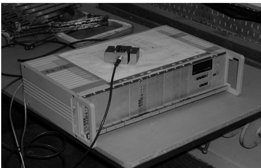
Figure D.8 8-channel amplifier used for the calibration of instruments
