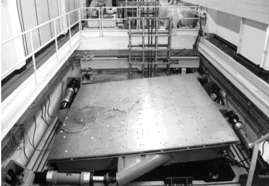
Figure D.1 Shaking-table at the University of Bristol facilities
