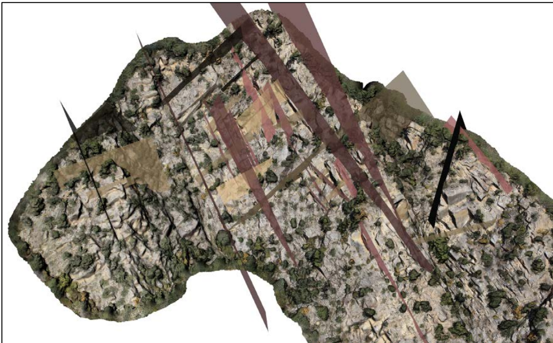
Figure 17: Manual modelling of joint sets by trace identification over 3D mesh texturized on Borrassica cliff (Andorra)
