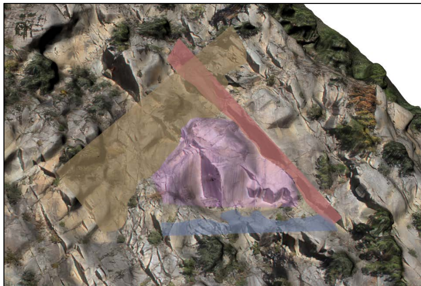
Fig. 6. Unstable rock mass delimitation based on 3D joints modeling.
