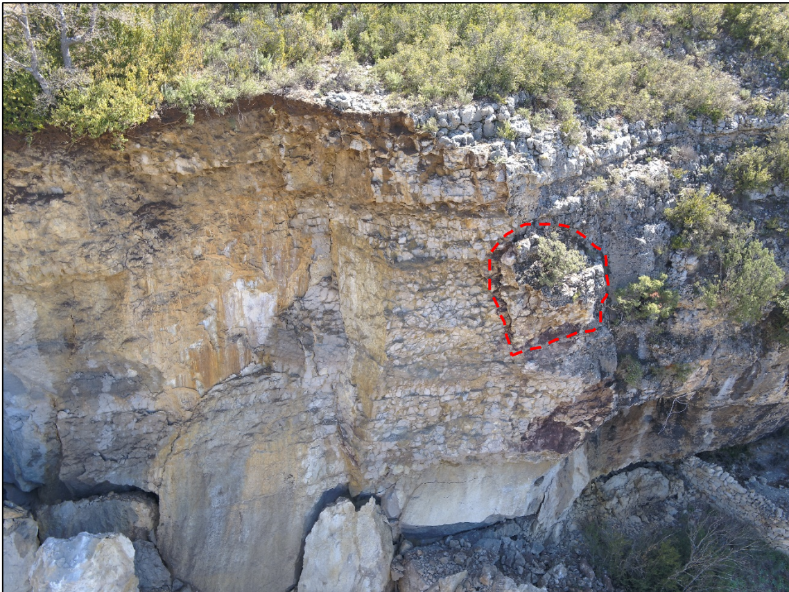
Figure 11: Up: Frontal orthophoto from Castell de Mur rockfall cliff obtained to identify unstable volumes. Down: Original picture from the drone (Castell de Mur rockfall) where an unstable rock mass can be identified.
