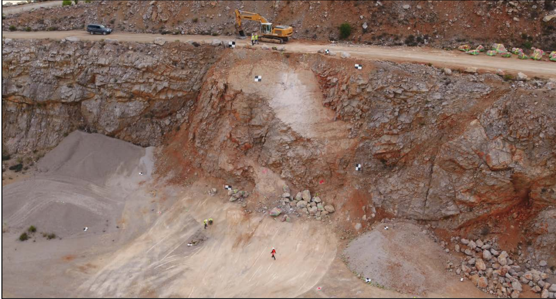
Figure 11: Picture of real-scale fragmentation test (test n° 4) performed in a limestone quarry.
