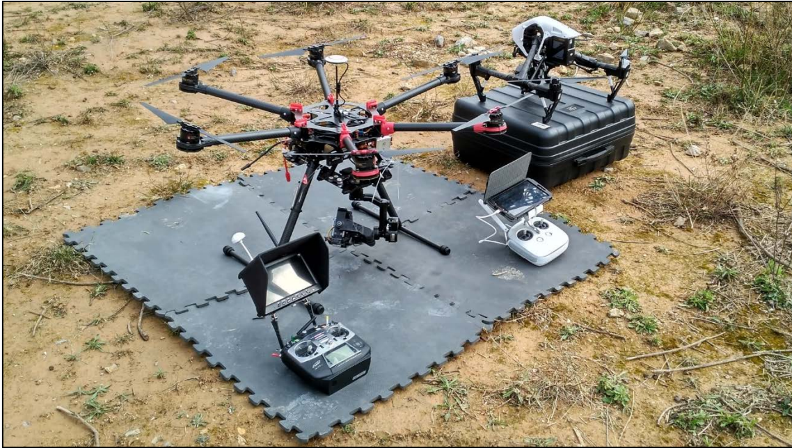
Figure 30: DJI-S900 self-mounted with a Sony NEX5 camera (left) and DJI-Inspire 1Pro with the camera X5 (right).
