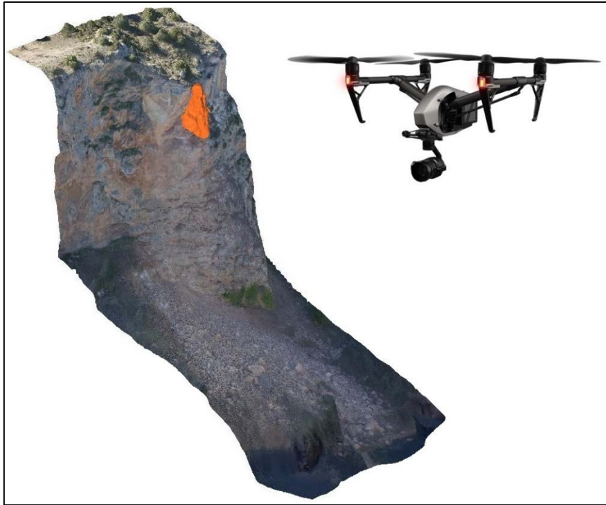
Figure 9: Texturized 3D model of a fragmental rockfall inventoried (Monasterio de Piedra), whereafter the rockfall event, an important unstable rock mass (orange volume) was characterized for further risk studies.
