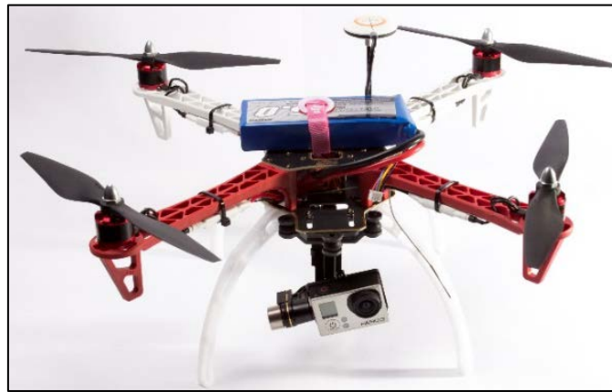
Figure 28: DJI F450 quadcopter mounted and used at the beginning of our research.
