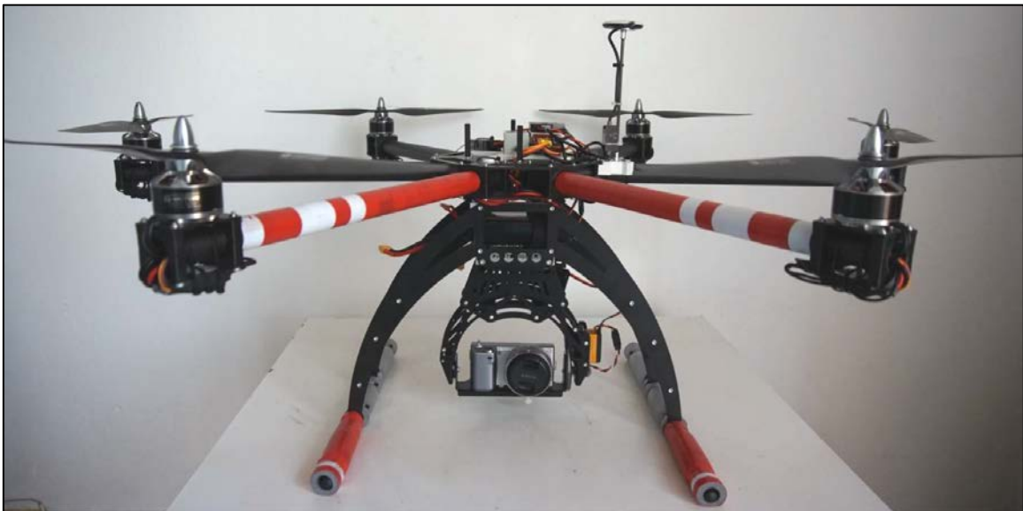
Figure 29: Self-constructed and based on our own design of a hexacopter (HexaCarbonFrame), in collaboration with Sjaedric Moreno Coscoll as designer, constructor and drone pilot.
