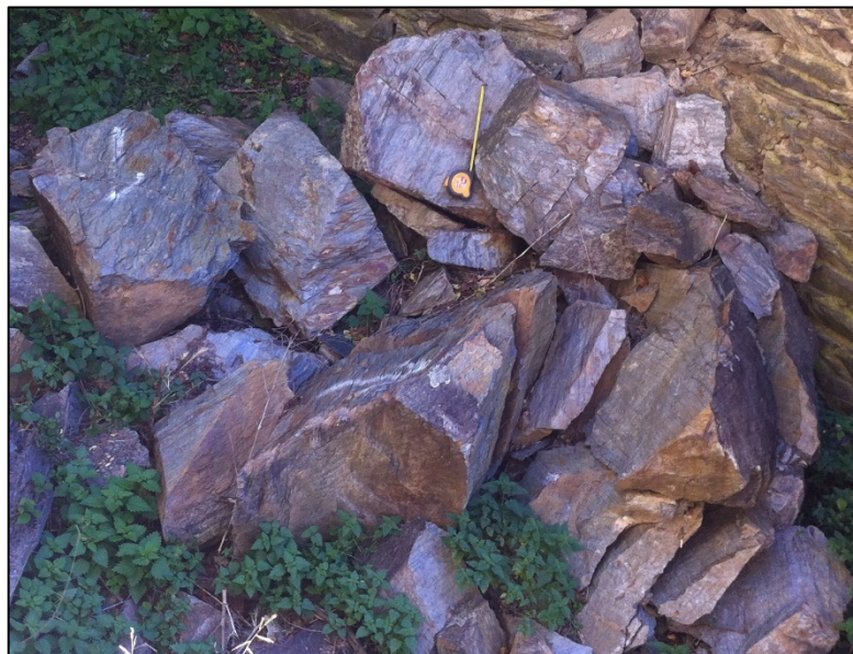
Fig.8: Example of a fragmental rockfall where the RBSD is very similar to the original IBSD. The rock mass was disaggregated along preexisting joint faces and no new fresh faces were generated by breakage
