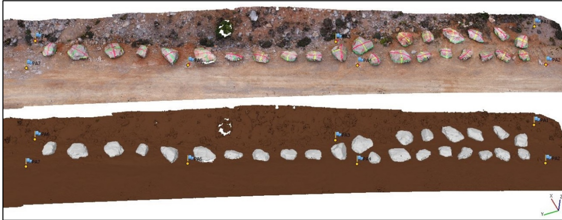
Figure 9: Blocks before test 4: Point cloud in real color (up) and point cloud classified in ground or not ground (down).
