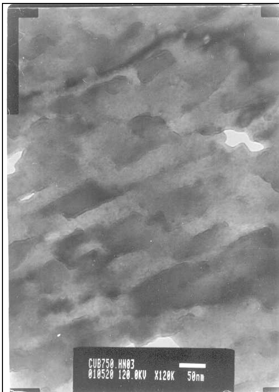
Fig. 3.69 A bright field TEM image of Cu B after 750°C, 0.3s^{-1} and \epsilon = 0.8 . The image only shows a flaky or grid like pattern.
