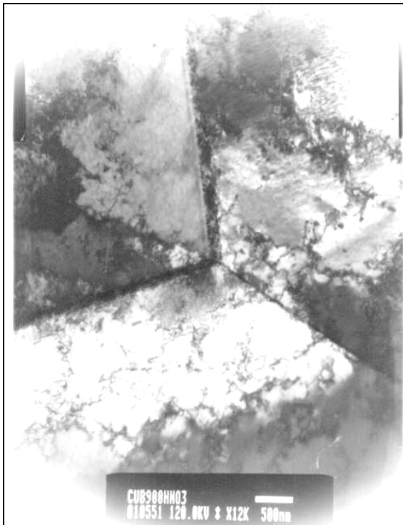
Fig. 3.76 The TEM foils from compressed samples after 900°C, 0.3s^{-1} and \epsilon = 0.8 did not show any precipitates, only regular images like above from Cu B where a triple junction grain boundary is seen with dislocations in contrast.
