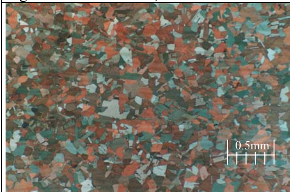
Fig. 3.39c After 800°C, 0.01s^{-1} and \varepsilon = 0.8 .
