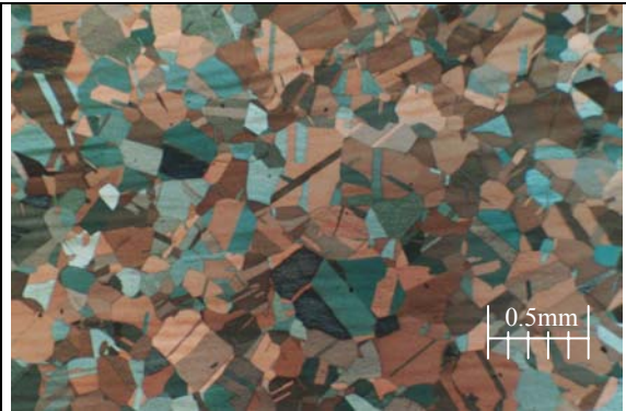
Fig. 3.42b After 950°C, 0.1s^{-1} and \varepsilon = 0.8 .
