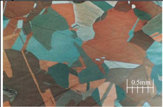
Fig. 3.42f After 950°C, 0.001s^{-1} and \varepsilon = 0.8 .
