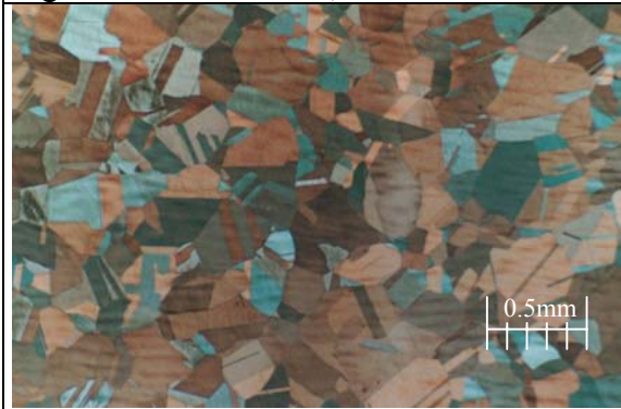
Fig. 3.42c After 950°C, 0.03s^{-1} and \varepsilon = 0.8 .
