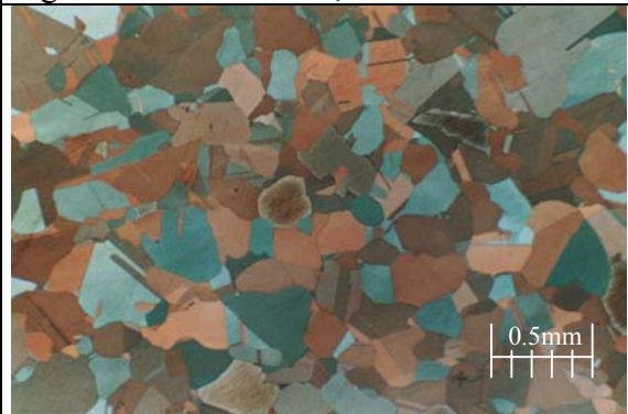
Fig. 3.40f After 850°C, 0.001s^{-1} and \varepsilon = 0.8 .
