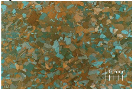
Fig. 3.37c After 700°C, 0.001s^{-1} and \varepsilon = 0.8 .
