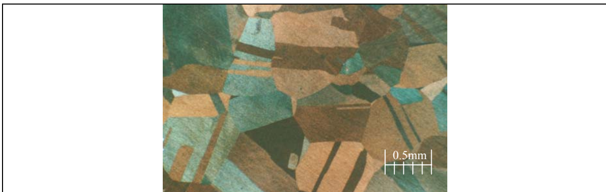
Fig. 3.33 Microstructure of Cu A after annealing, but before the hot compression tests.
