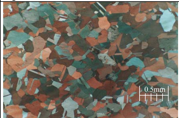
Fig. 3.39d After 800°C, 0.001s^{-1} and \varepsilon = 0.8 .
