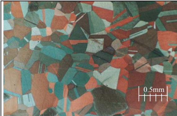
Fig. 3.42a After 950°C, 0.3s^{-1} and \varepsilon = 0.8 .
