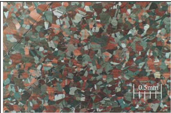
Fig. 3.40b After 850°C, 0.1s^{-1} and \varepsilon = 0.8 .
