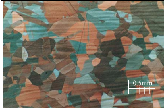
Fig. 3.42e After 950°C, 0.003s^{-1} and \varepsilon = 0.8 .
