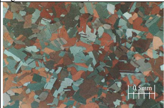
Fig. 3.38f After 750°C, 0.001s^{-1} and \varepsilon = 0.8 .
