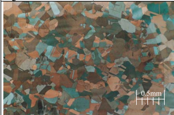
Fig. 3.40e After 850°C, 0.003s^{-1} and \varepsilon = 0.8 .
