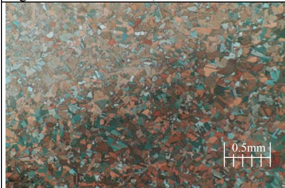
Fig. 3.38c After 750°C, 0.03s^{-1} and \varepsilon = 0.8 .
