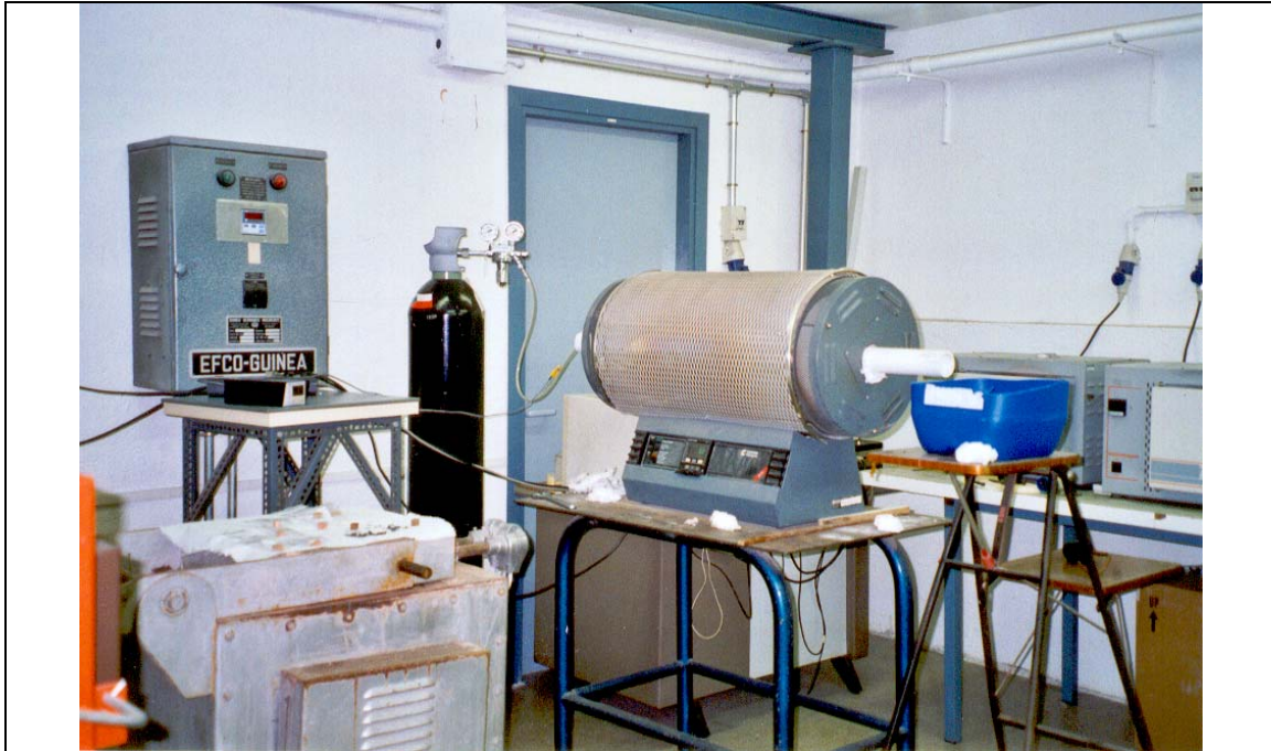
Fig. 2.6. Tube furnace and experimental setting used to perform the annealing treatments.
