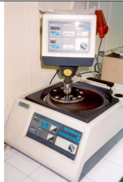
Fig. 2.18. Grinder-Polisher Ecomet 4 machine while polishing with diamond paste.
