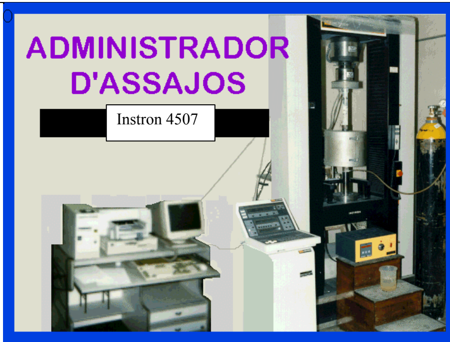
Fig. 2.7. A picture of the equipment used for hot compression testing: an Instron 4507 electromechanical testing machine, an inert gas flow system, a semi-electronically controlled temperature and a software “Administrador d’Assajos” to maintain a constant strain rate.
