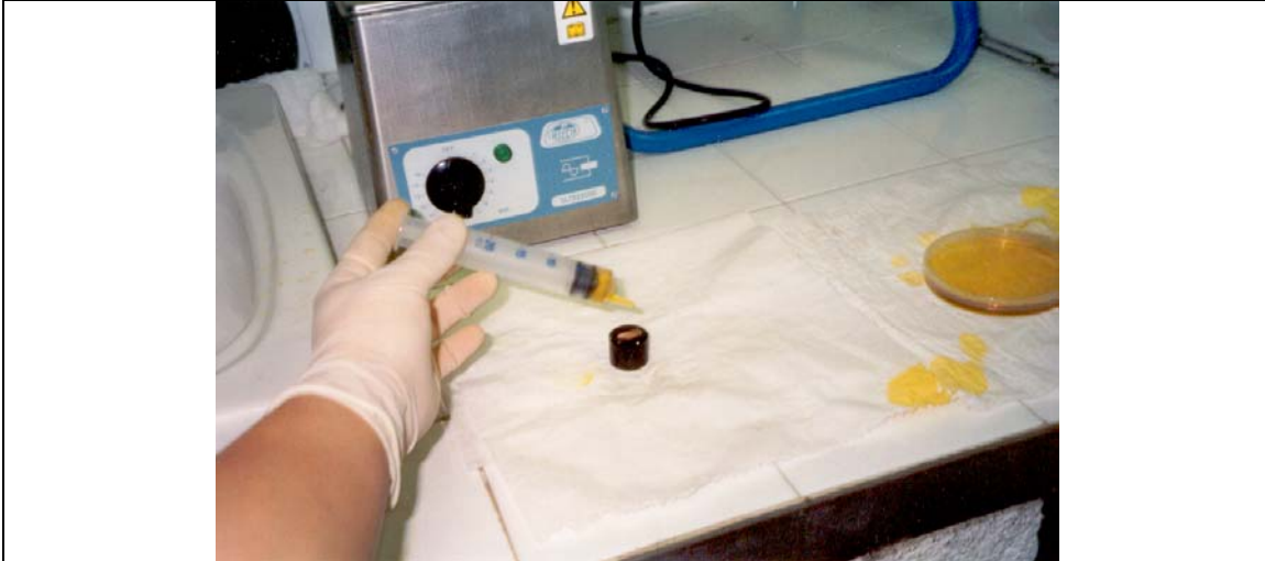
Fig. 2.19. A meniscus of distilled water was placed over the polished sample and three drops of etching acid were added as seen on the picture.
