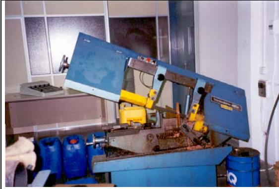
Fig. 2.4. Oil cooled band saw used to slice the copper surplus material.
