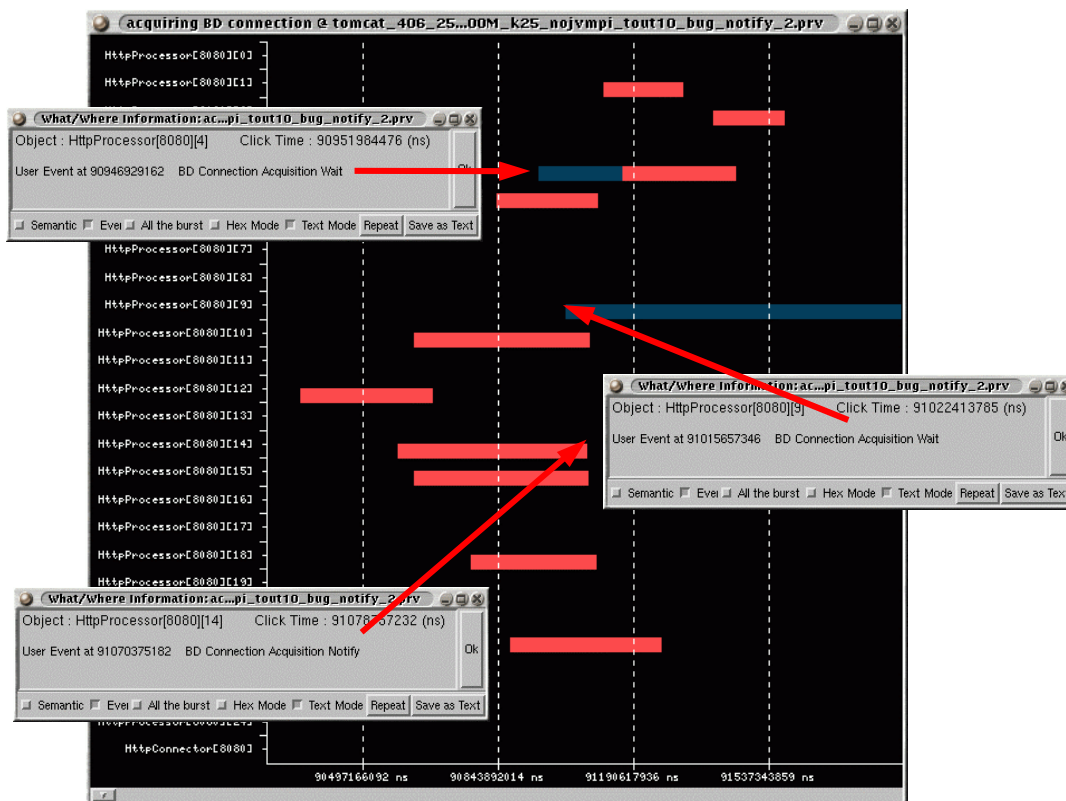
Figure 3.20. Database connections acquisition process
