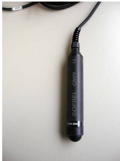
Figure 3.9: Type of water level sensor used in the Canal PAC-UPC
