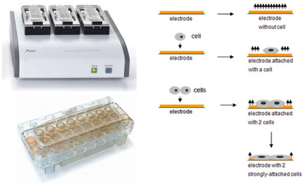
Figure XXI. xCELLigence System for monitoring cell adhesion.
