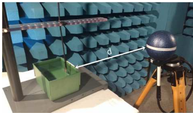
Figure 100. Experimental setup to measure the received electric field by the external isotropic antenna.
