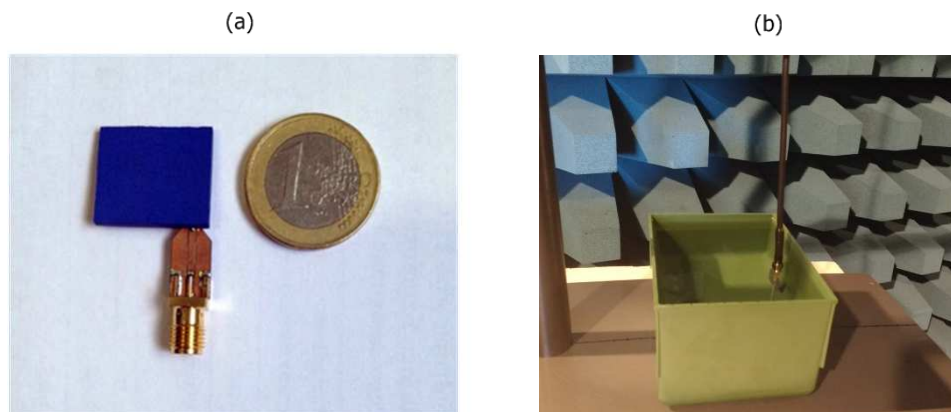
Figure 96. (a) Muscle tissue cuboid phantom used in simulations, (b) manufactured prototype in LTCC fed by a standard SMA connector through a coplanar wave guide launcher and (c) muscle tissue cuboid phantom used in the measurement setup.
