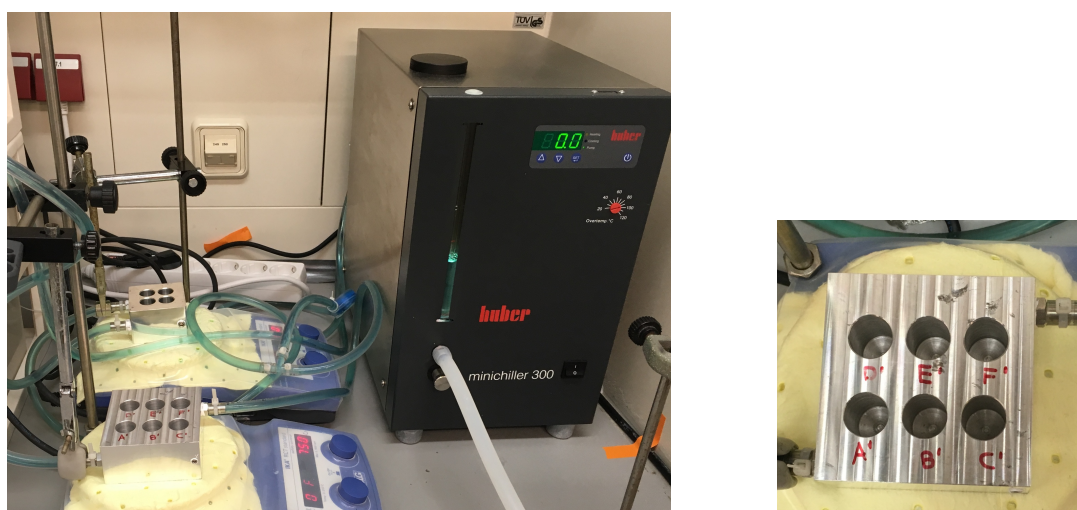
Figure 3.1. Laboratory set-up for low-temperature reactions
