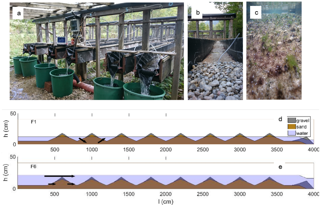
Figure 7.1: a) Flume outlets with discharge ascending from the left (F1) to the right (F6). b) Set up of flumes before water flow and c) underwater photo of biofilm after two weeks of treatment (17th of September 2015). d) Scheme of F1 during treatment with black arrows indicating the enforced water flow through the stream bed. e) Scheme of F6 during treatment with black arrows indicating the water flow predominantly above the stream bed.
