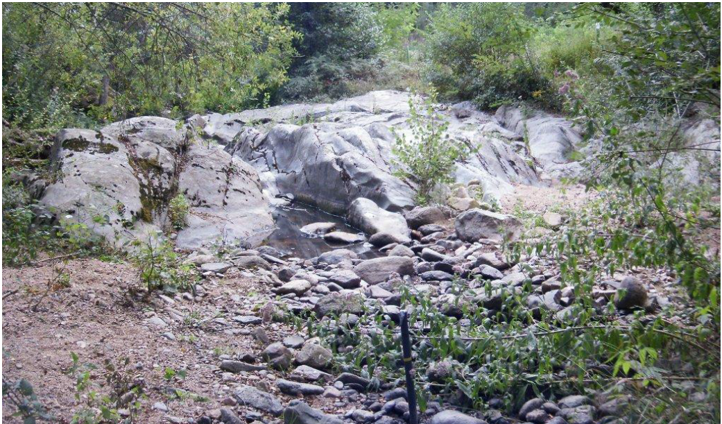
Figure 3.3: Photo of the study site (location see Figure 3.2). The uplift of the granitic bedrock is clearly visible in the back of the photo with the outlet of the pool. In the front part of the photo, a sampling well (HZ inf that is described in Chapter 3) installed in the alluvial sediments downstream of the pool.
