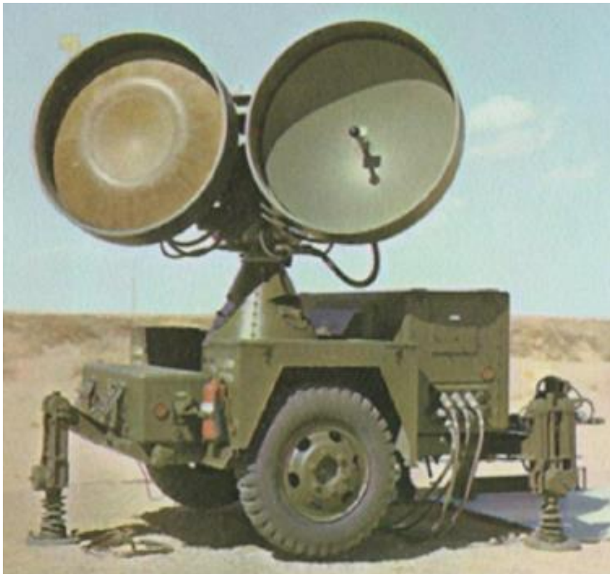
Figure 5. HAWK Low Power Illuminator military radar: frequency 10.25 GHz. Adapted from (Murata, Taichi K, 2015).
