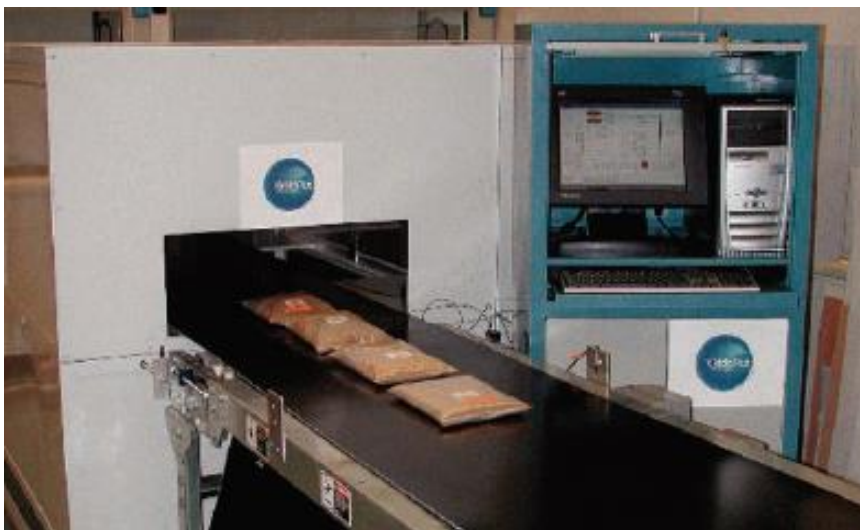
Figure 7. Intermediate frequency heating equipment for food disinfection. (Lagunas-Solar et al., 2006)
